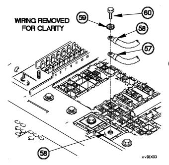
(29) Install terminal lug TL20 (10) on +24 VDC connector X1 (11) with lockwasher (9) and screw (8).
