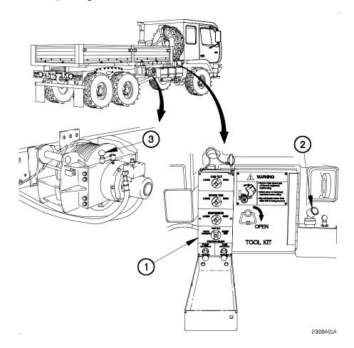
Figure 2-16. Passenger Side Exterior Controls
