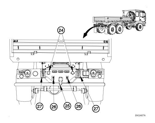
Figure 1-12. Common Vehicle Components Location (Cont)
