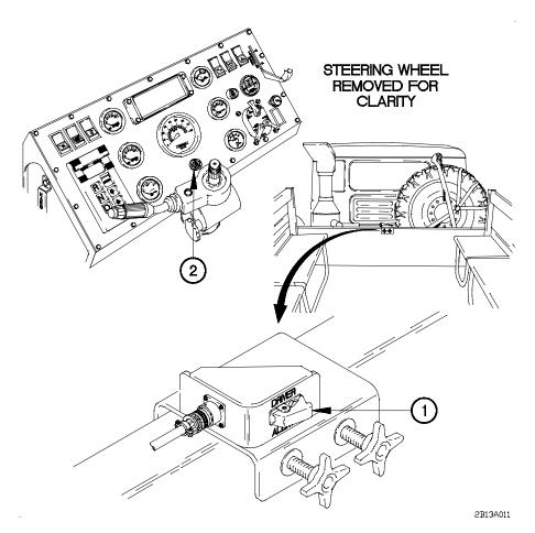
Figure 2-29. Troop Transport Alarm Switch
