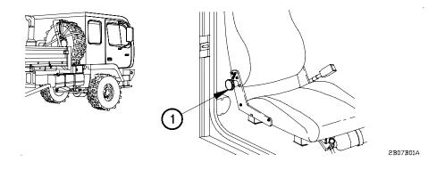
Figure 2-15. Right Passenger Seat Controls
