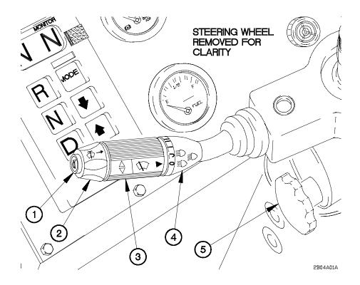
Figure 2-11. Steering Column Controls
