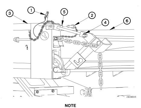
Both fixed links are removed the same way. Left side shown.
