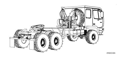
Figure 1-5. M1088 Truck, Tractor: 5-Ton, 6x6
