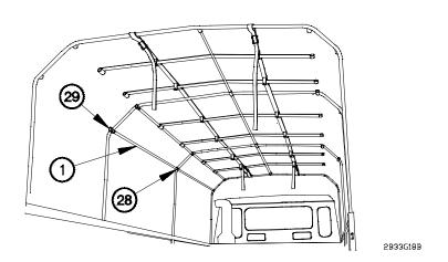
(38) Install center tube (1) in front center bow bracket (28) and rear center bow bracket (29).
