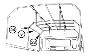
(31) Install front tube (8) in front bow bracket (23) and center bow bracket (24).
