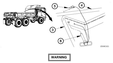
Cab protector is spring loaded and weighs approximately 180 lbs (82 kgs). Keep pressure on cab protector when lowering and when installing pins. Failure to comply may result in injury to personnel.
