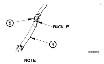
Front, front center, rear center, and rear bows have two bow straps and tiedown straps. All tiedown straps are installed on bow straps the same way. One tiedown strap shown.
