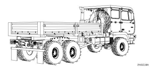
Figure 1-9. M1093 Truck, Cargo: 5-Ton, 6x6, Dropside, Air Drop
