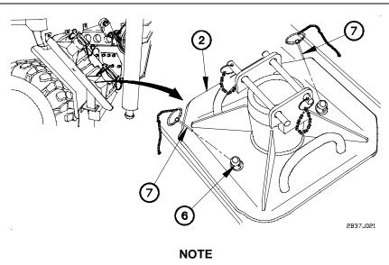
Both outrigger pads are installed on stowage bracket the same way.
