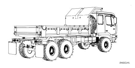
Figure 1-7. M1090 Truck, Dump: 5-Ton, 6x6
