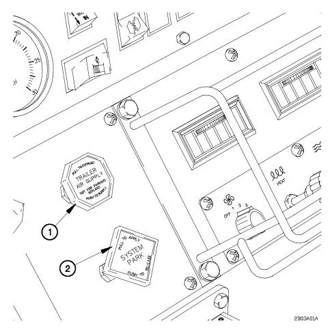
Figure 2-8. Air System Controls
