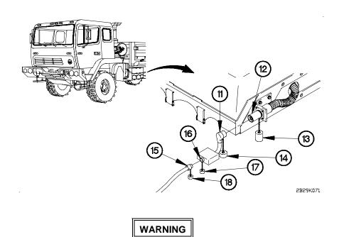
Ensure that engine is not running before disconnecting circuit breaker box NATO connector at vehicle NATO connector. Failure to comply may result in serious injury or death to personnel.
