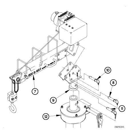
(9) Remove quick release pins (8 and 10) from turret (9).
