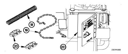
(17) Place spring (18), chain (19), and clamps (20) in tool box (22.1).
