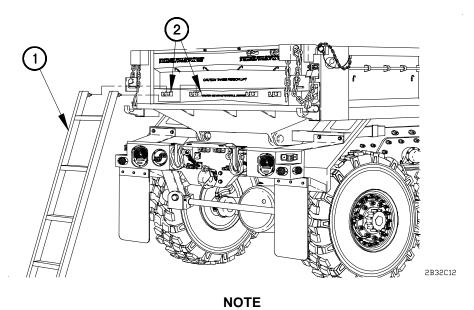
Perform step (5) to remove the ladder with the tailgate up.
