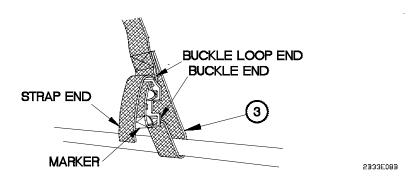
(19) Tighten left strap support (3) until marker is through the buckle end.
