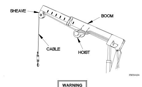
Wear heavy leather-palmed work gloves when handling cable. Cables can become frayed or contain broken wires. Never let moving cable slide through hands, even when wearing gloves. Failure to comply may result in injury to personnel.
