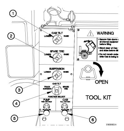
Figure 2-17. Hydraulic Manifold Controls
