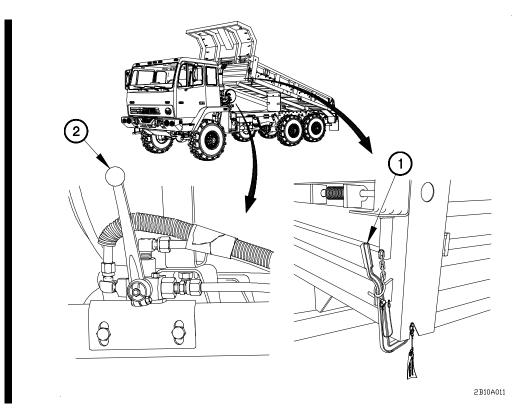
Figure 2-22. Exterior Dump Body Controls
