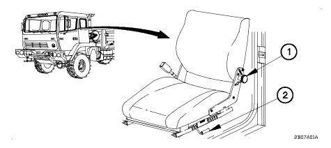
Figure 2-14. Driver's Seat Controls
