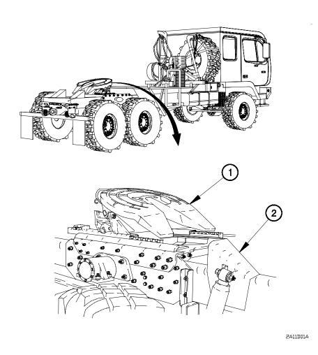
Figure 1-15. M1088 Tractor Components Location
