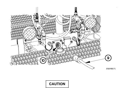
After disconnecting intervehicular cable, close the receptacle cover. Failure to comply may cause damage to equipment.
