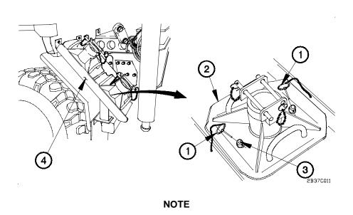
Both outrigger pads are removed the same way. Left side shown.
