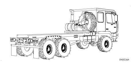
Figure 1-8. M1092 Truck, Chassis: 5-Ton, 6x6
