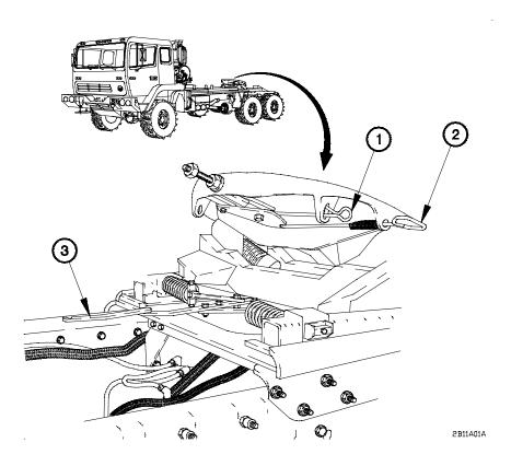
Figure 2-23. Tractor Fifth Wheel Controls
