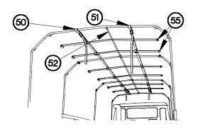
(56) Remove two braces (55) from rear tube (52), left strap support (50), and right strap support (51).
