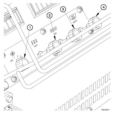
Figure 2-9. Heater/Defrost Controls
