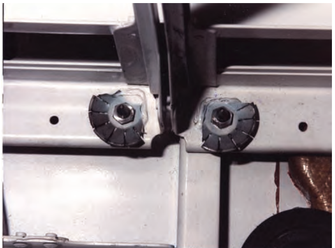
Figure 6-5. EMI Bonding Washers in Avionics Bay
