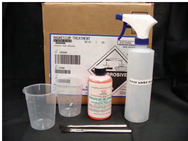
Figure 5-4. Magnesium Treatment Kit
