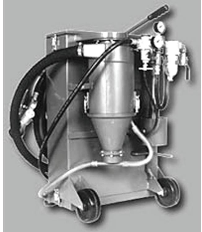
Figure 4-6. Portable Vacuum Blast Equipment
