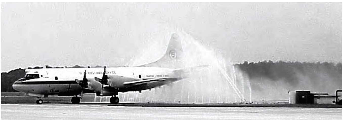
Figure 2-7. Aircraft at a Taxi-Through Rinse Facility
