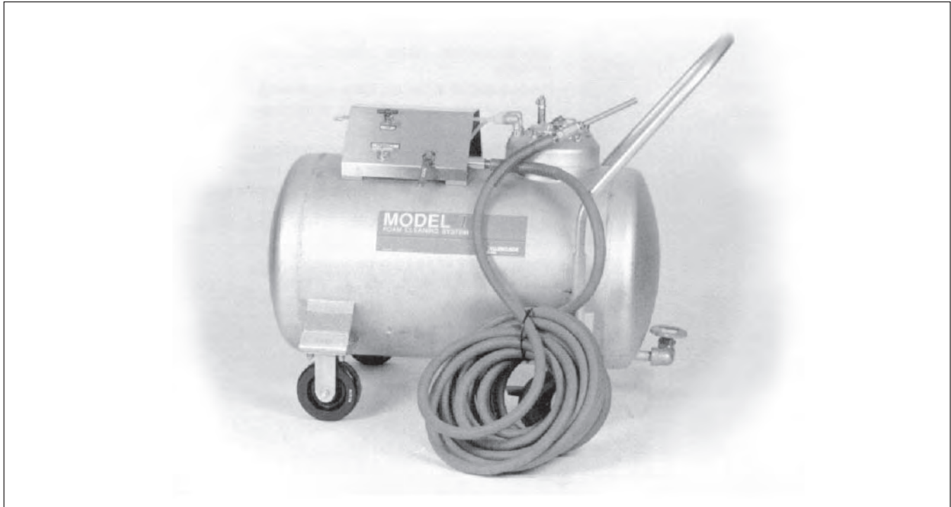
Figure 2-2. Large Portable Foam Generating Cleaning Unit (45 Gallons)
