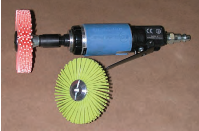
Figure 4-2. Bristle Discs Stacked on Mandrel Assembly
