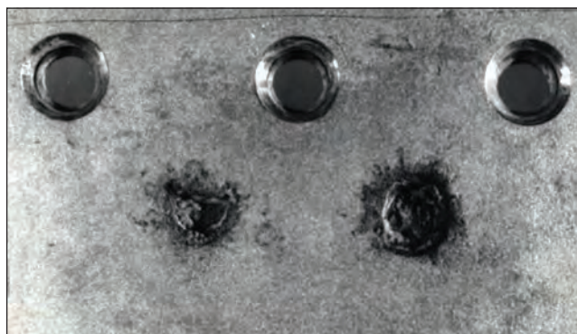
Figure 3-20. Spot Weld Corrosion
