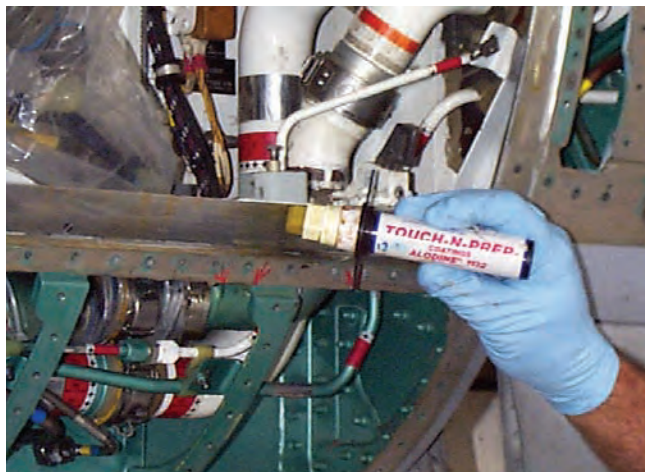
Figure 5-3. Application of TNP Pen on Aluminum Substrate
