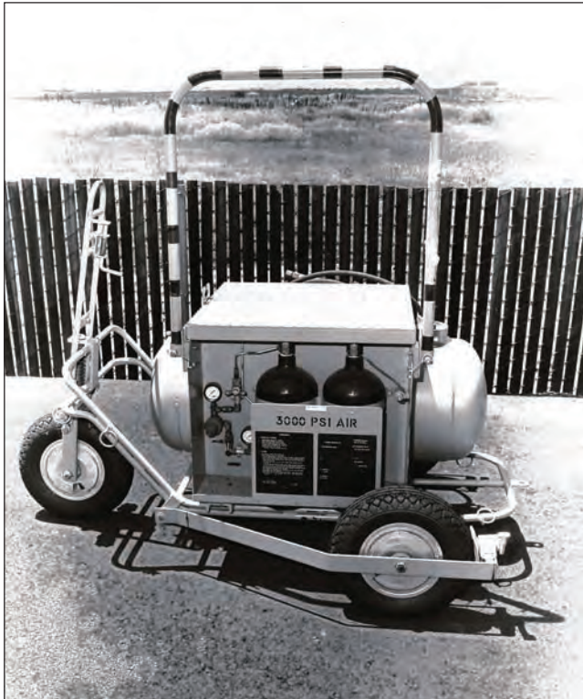
Figure A-18. Jet Engine Corrosion Control Cart
