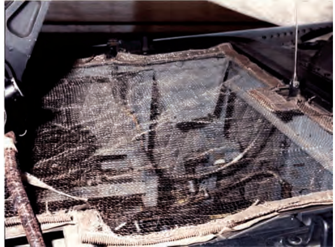
Figure 6-3. Stainless Steel EMI Screen
