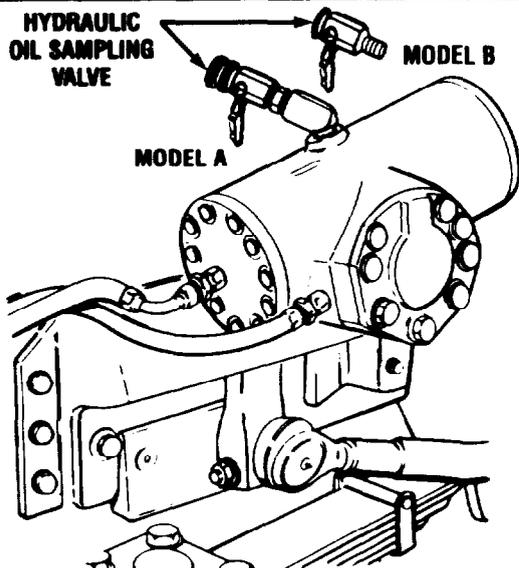
SLAVE STEERING GEAR OIL SAMPLING VALVE
