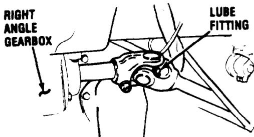
U-JOINT—RIGHT ANGLE GEARBOX TO FIRST STEERING SHAFT
