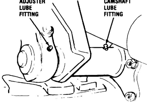
**NO. 3 AND 4 AXLE BRAKE CAMSHAFT AND
