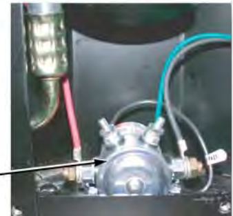
AC CONDENSER MOTOR SOLENOID
