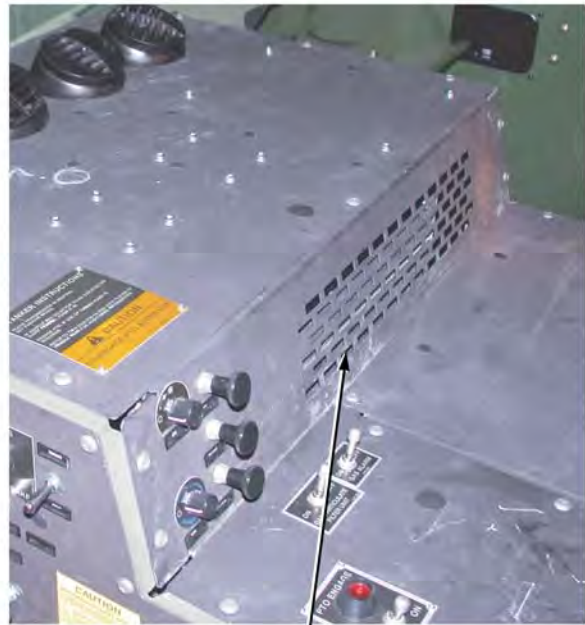
INTAKE VENT AND AC HEATER/EVAPORATOR CORE
