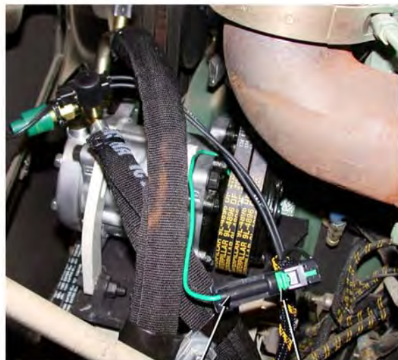
AC COMPRESSOR CLUTCH CONNECTOR
