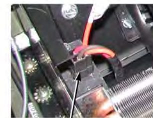
AC HEATER/EVAPORATOR BLOWER MOTOR RESISTOR HARNESS CONNECTOR
