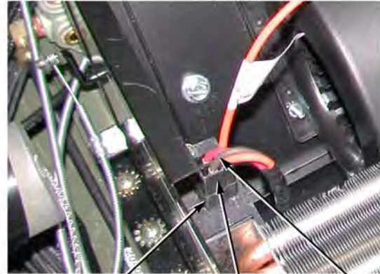
AC HEATER/EVAPORATOR BLOWER MOTOR RESISTOR AC HEATER/EVAPORATOR BLOWER MOTOR RESISTOR HARNESS CONNECTOR BROWN WIRE
