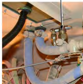
SYSTEM LOW-SIDE AC HOSE (AC EVAPORATOR CORE OUTPUT)
