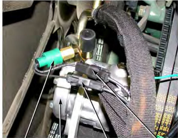
HIGH PRESSURE SWITCH AC COMPRESSOR HIGH PRESSURE SWITCH WIRE 1158 CONNECTOR HIGH PRESSURE SWITCH WIRE 1156 CONNECTOR
