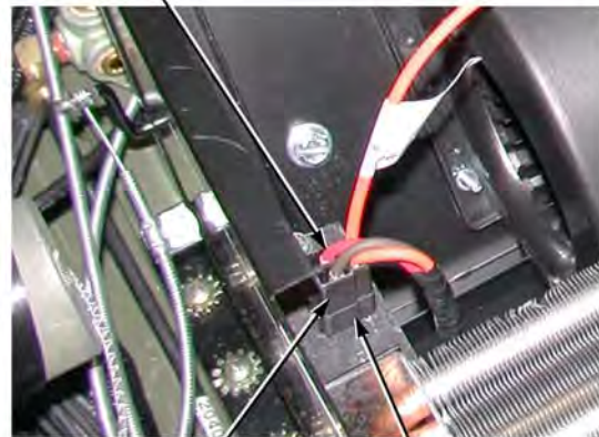
AC HEATER/EVAPORATOR BLOWER MOTOR RESISTOR HARNESS CONNECTOR
