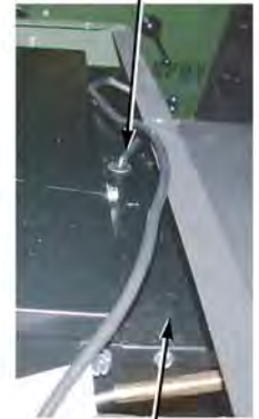
AC HEATER/EVAPORATOR CORE COVER
