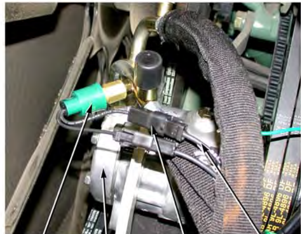
HIGH PRESSURE SWITCH AC COMPRESSOR HIGH PRESSURE SWITCH CONNECTOR AC HARNESS WIRE 1156
