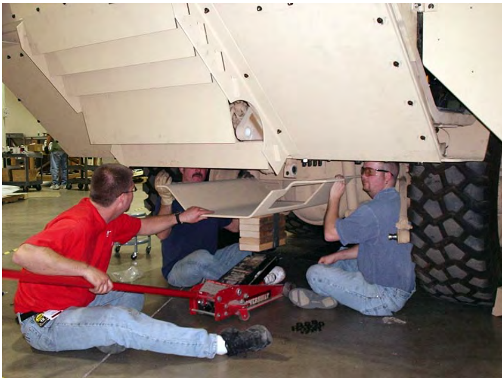
Figure 31. Position the Center Blast Deflector onto the Mounting Bracket Studs.
