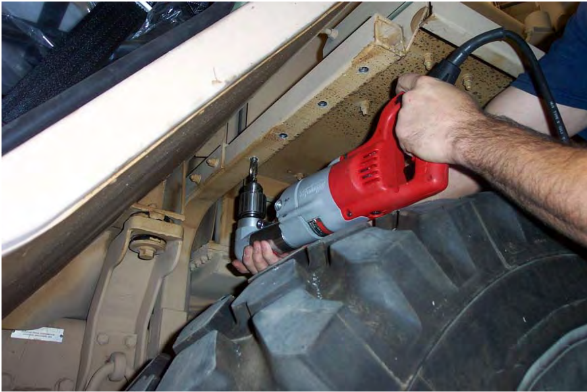
Figure 37A. Drill the holes for the Front Blast Deflector in the bottom of the fender support.
