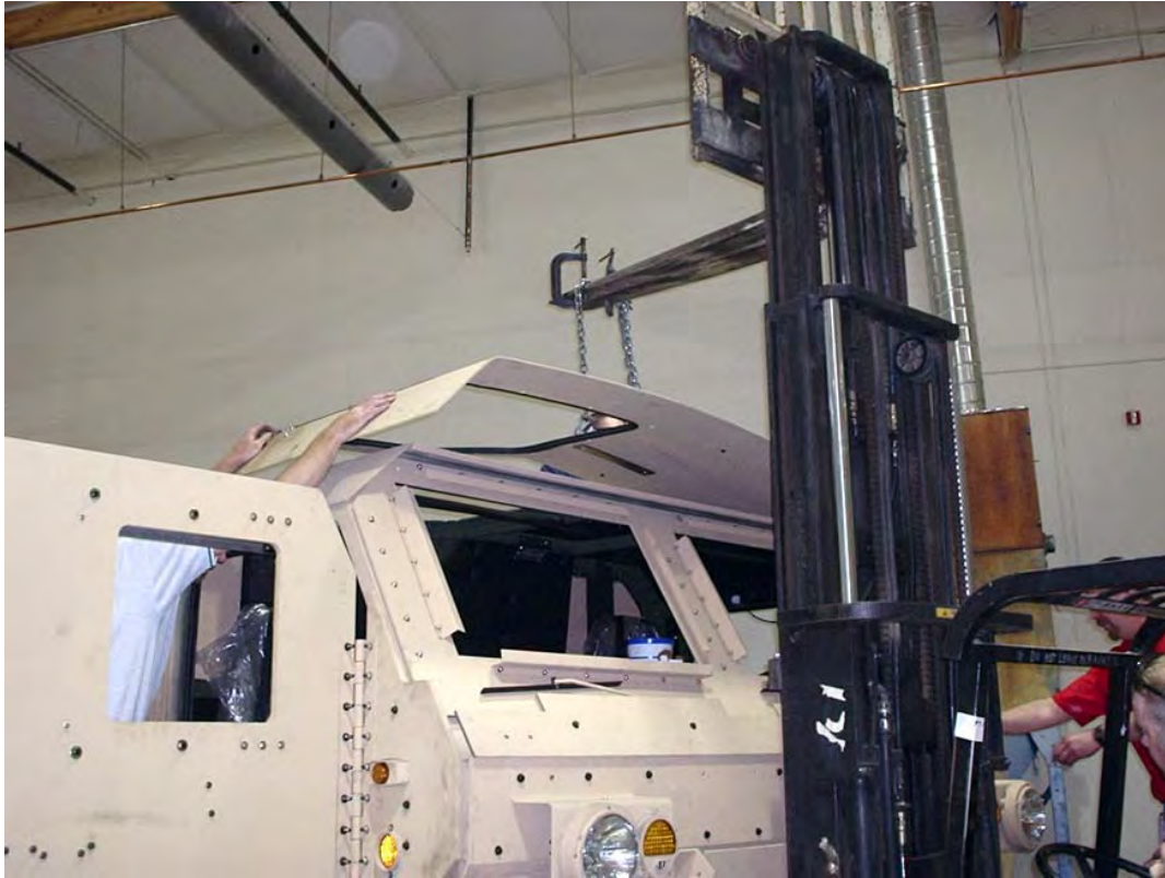
Figure 46. Lift the Roof Armor Panel into place on the HEMTT roof.
