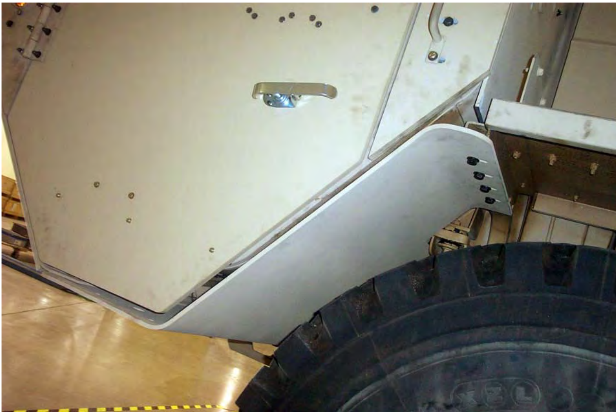
Figure 38. Install the driver's-side front blast deflector (P/N 106717-1).
