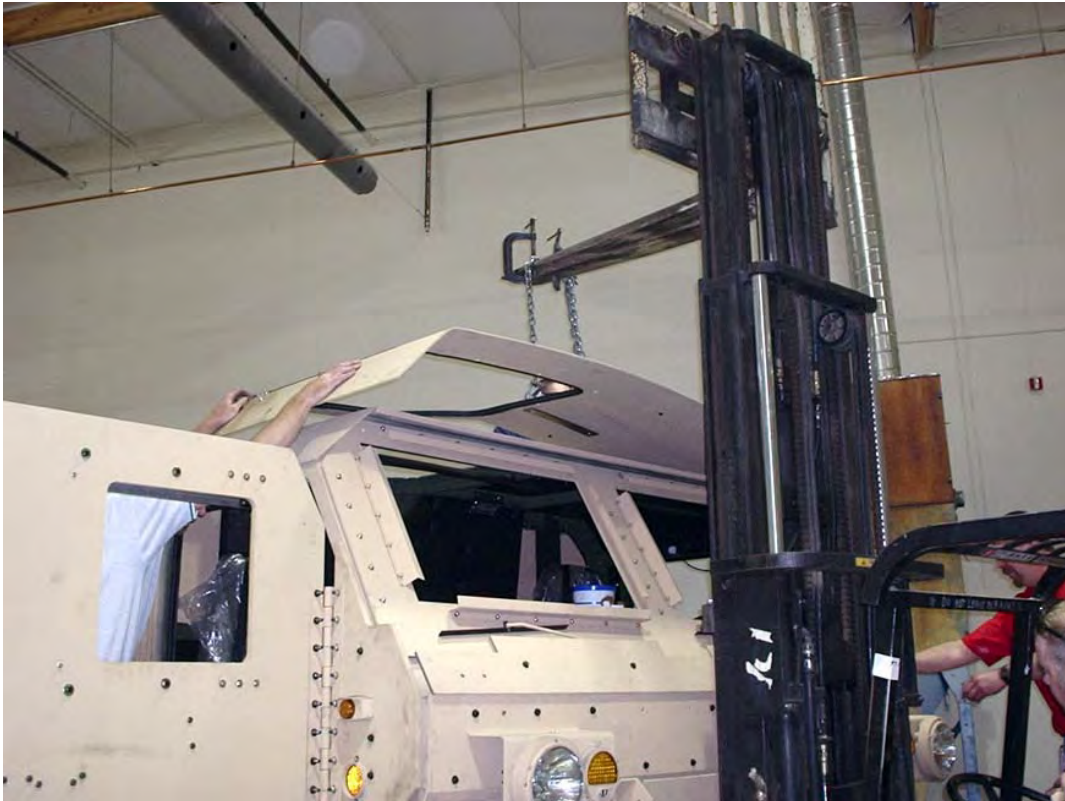
Figure 41. Lift the Roof Armor Panel into place on the HEMTT roof.
