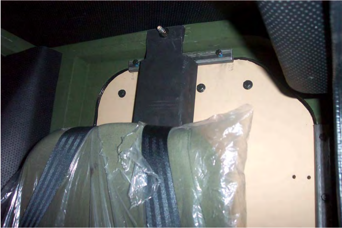
Figure 26. Move the Harness Bracket to the inside for increased clearance for the Rear Cab Armor Panel Bracket.
