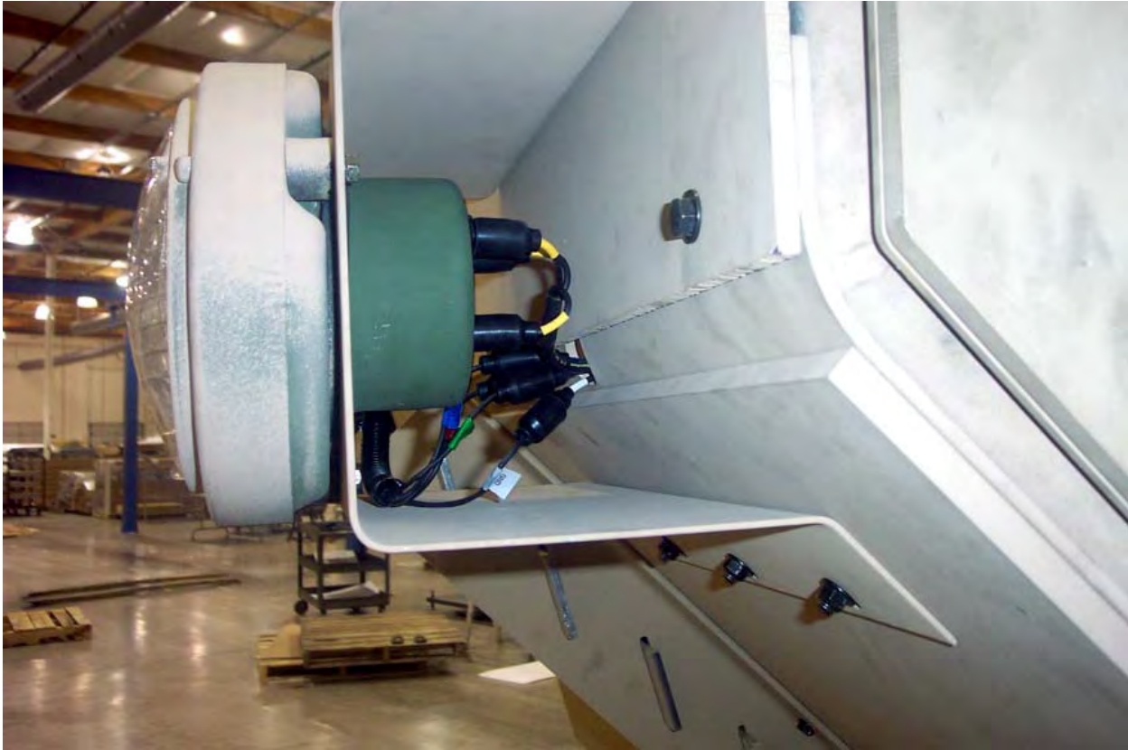
Figure 25. Left-hand Headlight Bracket Installed.
