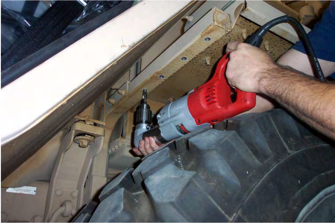
Figure 30a. Drill the holes for the Front Blast Deflector in the bottom of the fender support.
