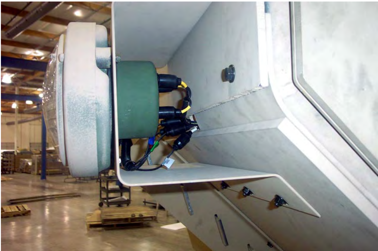
Figure 28. Left-hand Headlight Bracket Installed.
