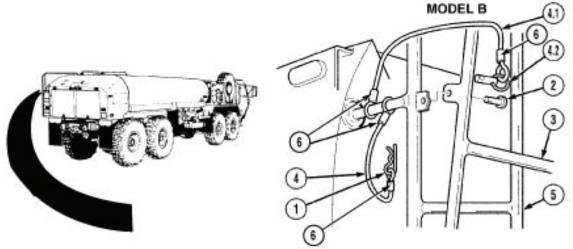
Remove pin (2) and deploy lower ladder assembly (3).
