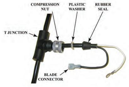
7. Route black wire and white wire through compression fitting on driver side compartment light base, and install compression nut on compression nut base.
