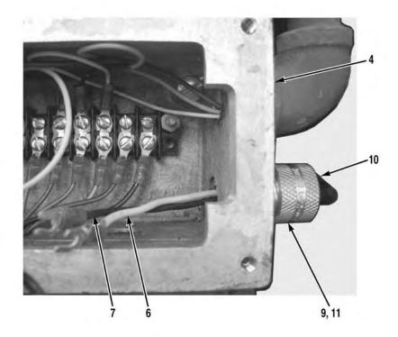
3. Loosen compression nut (9). Remove cable (10), white wire with brown tape (6), black wire (7), plastic washer (11), and compression nut (9) from control junction box (4).
