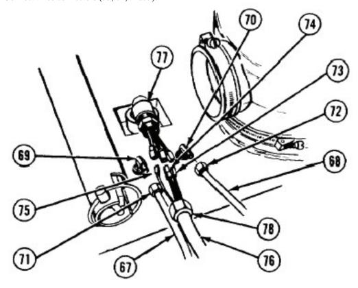
Install hose (76) on tank level sensor (77) with nut (78).
