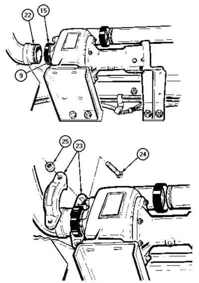
Install two coupling halves (23) with screws (24) and nuts (25).
