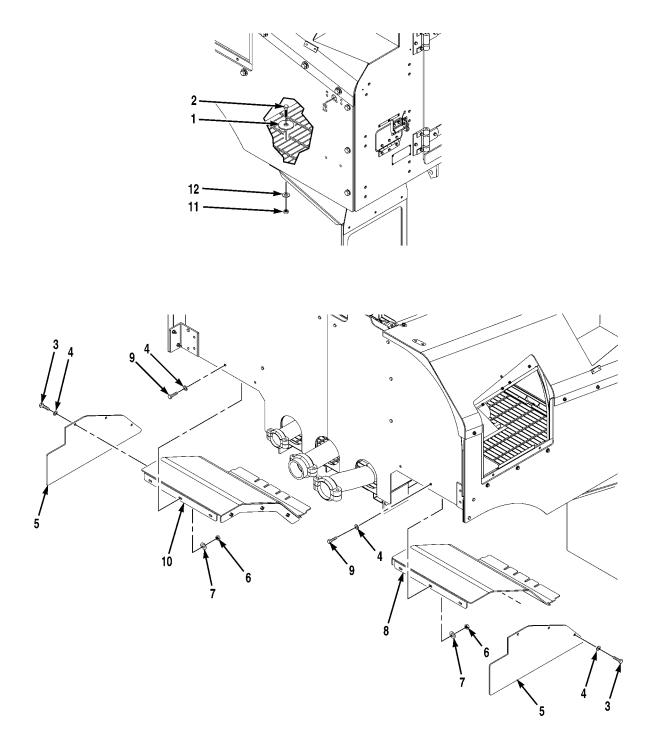
FIG. 7 WHEEL WELL ASSEMBLY
