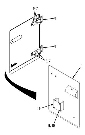
1. Remove four screws (6), lockwashers (7), and two rear door hinges (8) from rear door assembly (1). Discard lockwashers.
