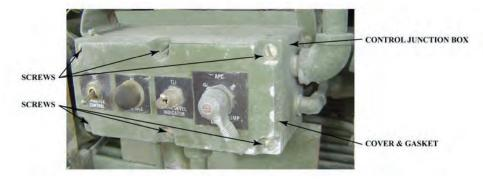
3. Loosen two screws, and the brown wire and black wire from the elbow, from terminal board.
