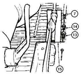
Install fitting (13) and nut (14) in frame (15). Do not tighten fitting. Install cable (7) through nut (14) and fitting (13). Tighten nut (14).
