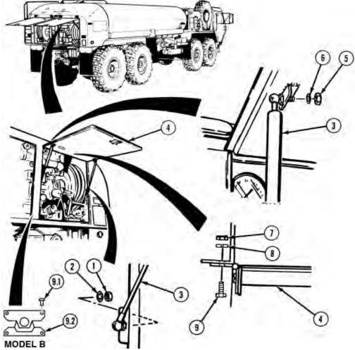
Remove nuts (5) and lockwashers (6) from upper end of both push rods (3). Remove eight nuts (7), lockwashers (8), and screws (9). Remove door (4).
