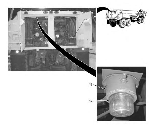
14. Install compartment light lens (12) on compartment light base (13).
