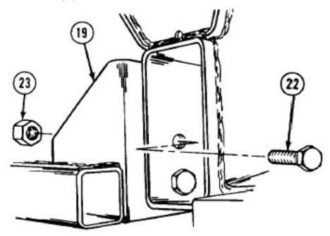
Soldier A installs two screws (22) in left side of tank front crossmember (19) while Soldier B installs and holds nuts (23).
