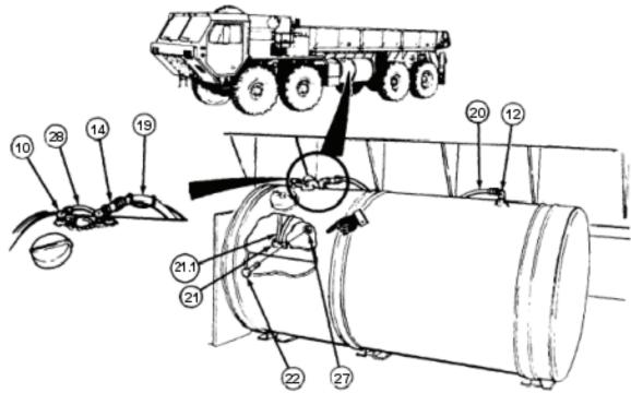
Coat threads of check valve (14) and elbow (12) with pipe thread sealing compound.
