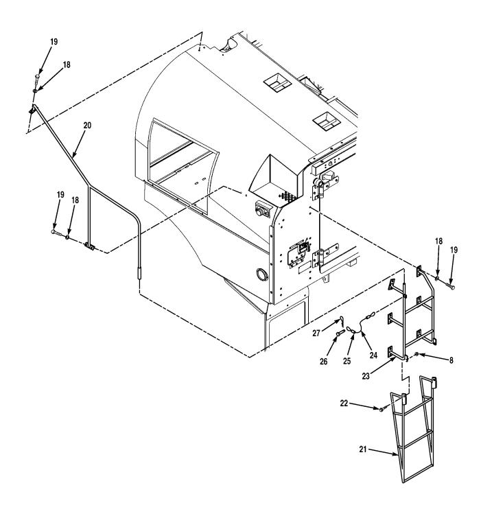
FIG. 9 LADDERS AND BRACKETS (SHEET 2 OF 3)
