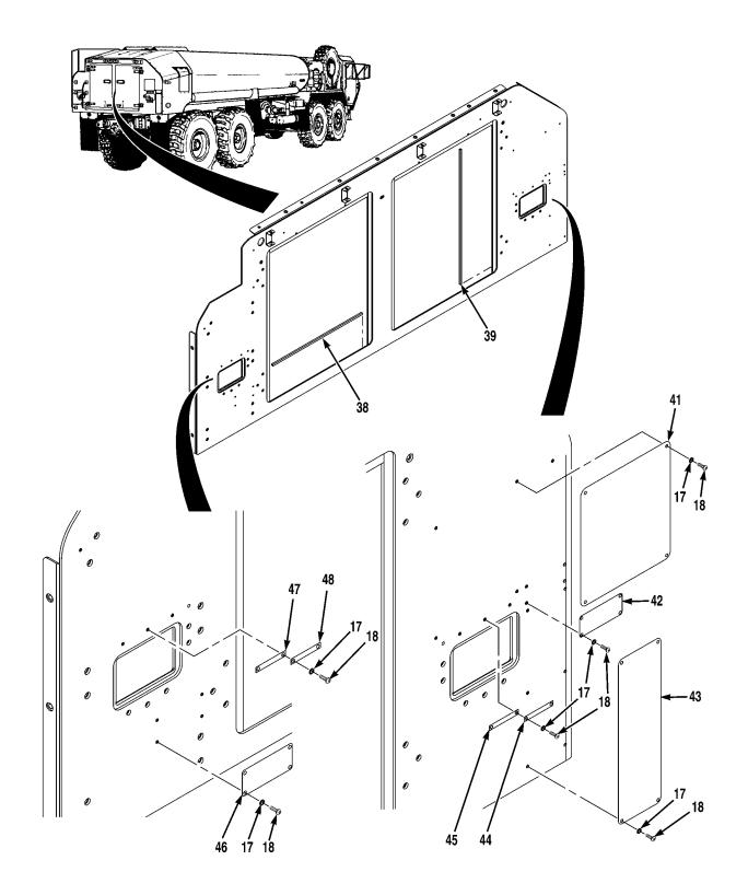
FIG. 1 REAR PANEL ASSEMBLY (SHEET 3 OF 3)
