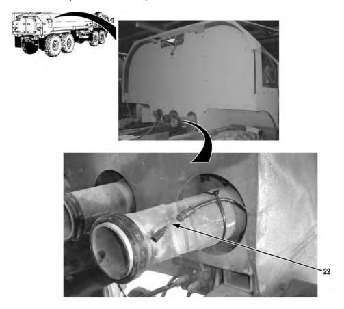
15. Connect tank connector (22) to existing chassis harness.
