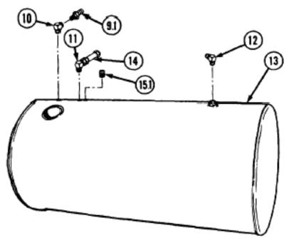
Coat air vent (10) and two elbows (11 and 12) with pipe thread sealing compound and install elbows in fuel tank (13).
