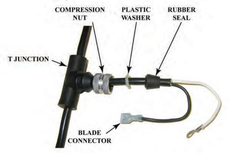
9. Route black wire and white wire through compression fitting on driver side compartment light base, and install compression nut on compression nut base. A2 model shown; previous models similar.
