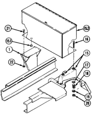
Install plug (15.1) into stowage box (15.2). Soldier A operates lifting device while Soldier B aligns mounting bracket (1) and rubber mounts (15). Install two screws (16), washer (17), spring (18), washer (19), and two nuts (20). Soldier A installs four screws (21) while Soldier B installs four locknuts (22).
