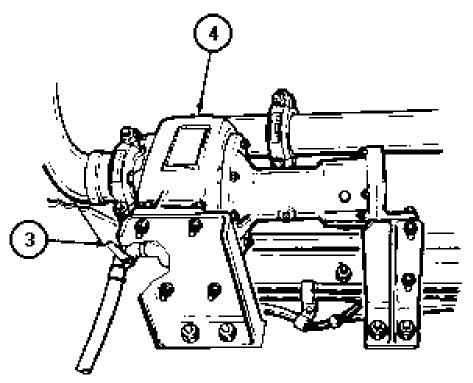
29. Open drain valve (3) on primary pump (4) and drain remaining fuel.
