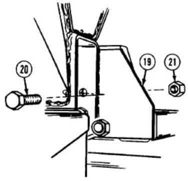
Soldier A installs three screws (20) in right side of tank front crossmember (19) while Soldier B installs and holds nuts (21).
