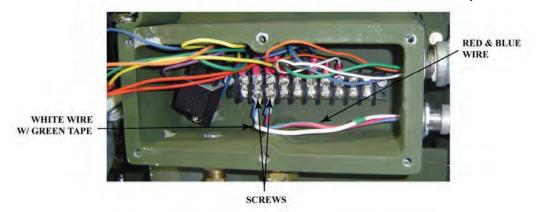
4. Loosen compression nut. Remove cable, wires, rubber seal, plastic washer, and compression nut from control junction box.
