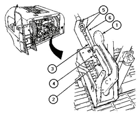
Remove nut (2) and cable (3) from offset link (4). Loosen two nuts (5) and remove cable (3) from bracket (6).
