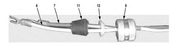
4. Remove rubber seal (11), plastic washer (12), and compression nut (9) from white wire with green tape (6) and red and blue wire (7).
