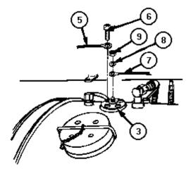
Install wire (7) with lockwasher (8) and nut (9) on fuel level sending unit (3).
