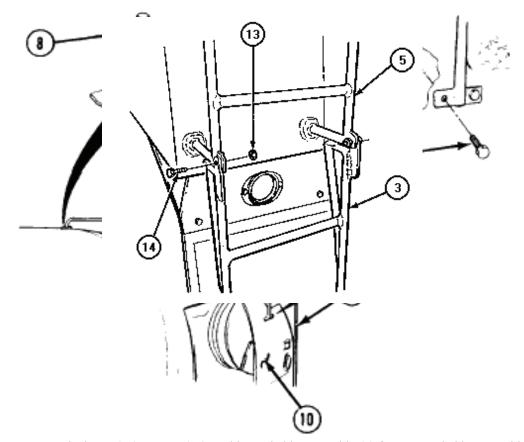
Remove two locknuts (13), screws (14), and lower ladder assembly (3) from upper ladder assembly (5).
