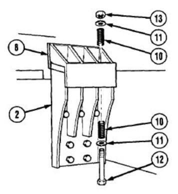
Install six springs (10), washers (11), three screws (12), and locknuts (13) in front tank mounting bracket (8) and frame mounting bracket (2).
