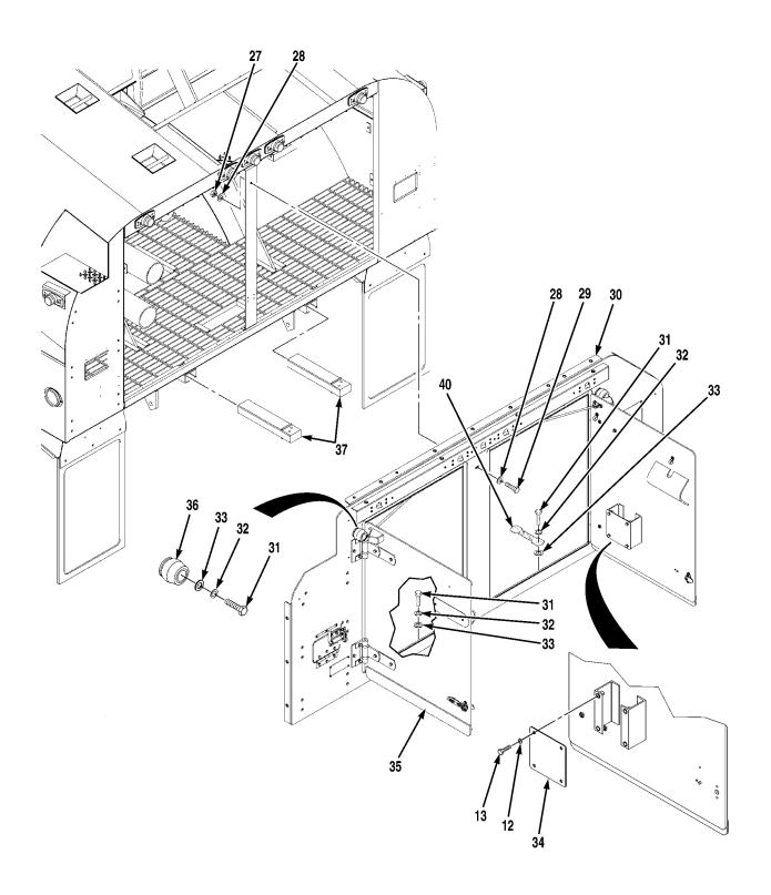
FIG. 1 REAR PANEL ASSEMBLY (SHEET 2 OF 3)
