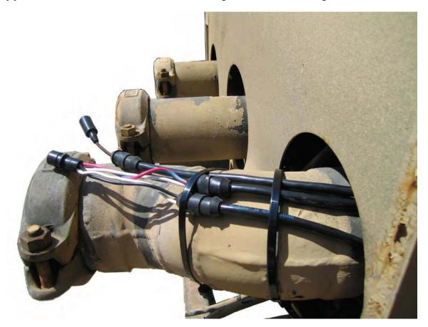
16. Secure all loose cables to existing hardware with cable ties.
