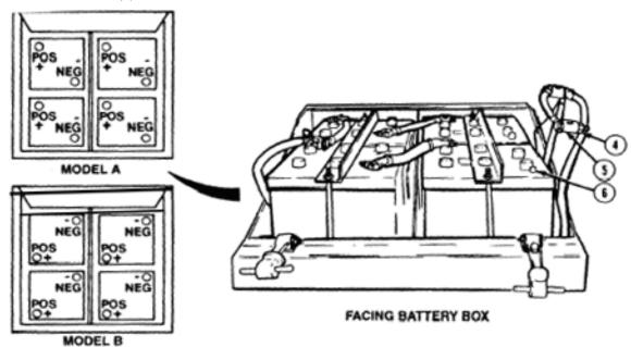
Disconnect two negative cable terminals (5) from battery posts (6).
