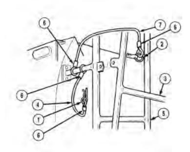
Remove pin (2) and deploy lower ladder assembly (3).
