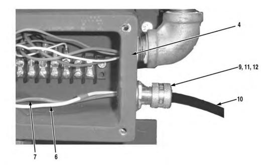
3. Loosen compression nut (9). Remove cable (10), white wire with green tape (6), red and blue wire (7), rubber seal (11), plastic washer (12), and compression nut (9) from control junction box (4).
