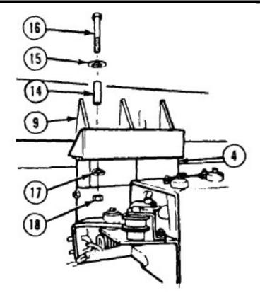
Install four spacers (14), washers (15), screws (16), washers (17), and locknuts (18) in rear tank mounting bracket (9) and frame mounting bracket (4). Do not tighten locknuts.
