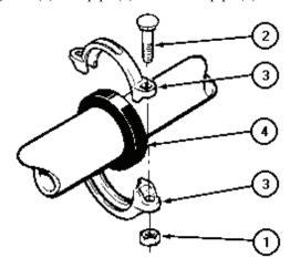
Remove coupling gasket (4) from pipe.
