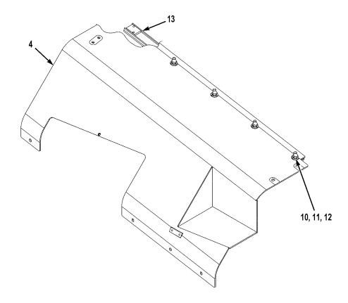
1. Remove five screws (10), lockwashers (11), washers (12), and one tapping channel assembly (13) from left upper side panel assembly (4). Discard lockwashers.
