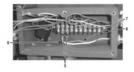
2. Loosen two screws (5) and remove white wire with green tape (6) and red and blue wire (7) from terminal board (8).
