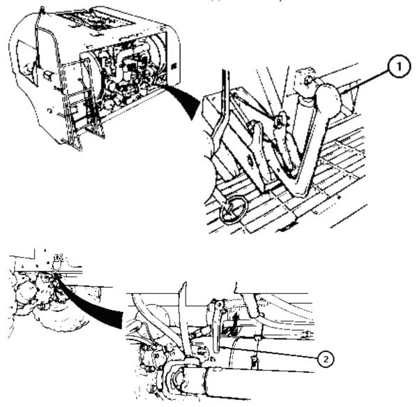
2. Set V3 suction line valve handle (2) to OPEN position.
