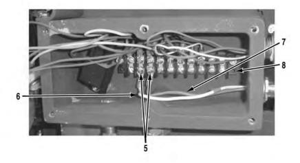
4. Install white wire with green tape (6) and red and blue wire (7) on terminal board (8) with two screws (5).
