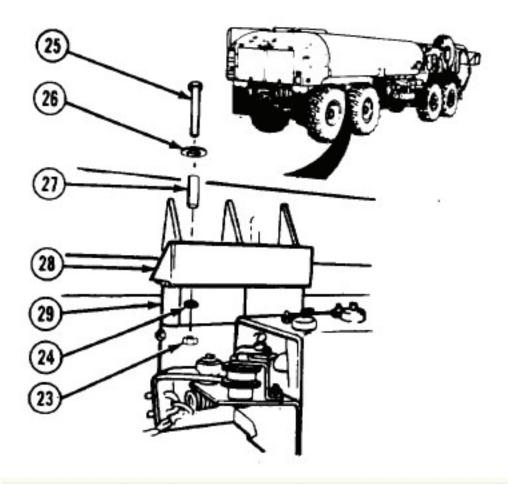
Tank must be lifted slowly and carefully. Make sure no wires, hoses, or linkages are caught during removal, or severe damage to tank and chassis will result.
