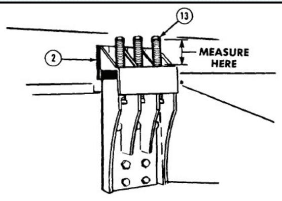
Tighten three locknuts (13) on front tank mounting brackets (2). Tighten four locknuts (18) on rear frame mounting brackets (4). Torque to 150 lb-ft (203 N•m).
