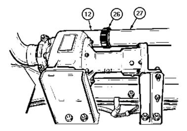
Position coupling gasket (26) over ends of discharge elbow (12) and discharge pipe (27).
