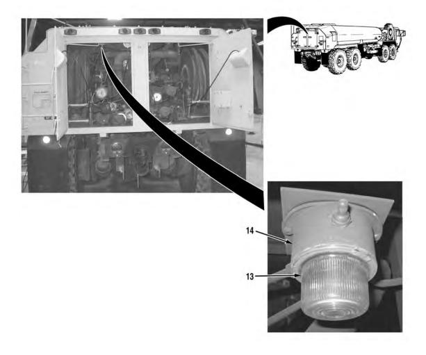
12. Install compartment light lens (13) on compartment light base (14).
