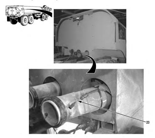
13. Connect tank connector (23) to existing chassis harness.
