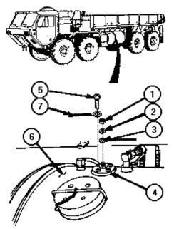
Remove one screw (5) holding fuel level sending unit (4) to fuel tank (6). Remove ground wire (7).
