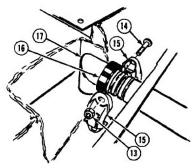
Push coupling gasket (16) onto pipe (17).
