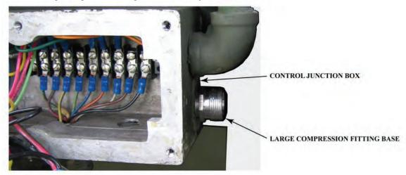
3. Test-fit smaller compression fitting in forward center hole of driver side compartment light base. If the compression fitting can be installed, proceed to step 5. Bulb shown removed for clarity.
