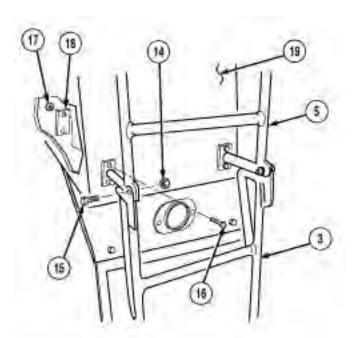
Remove two locknuts (14), screws (15), and lower ladder assembly (3) from bolt-on ladder assembly (5). Remove 12 screws (16), locknuts (17), and six mounting plates (18) from pump module panel (19) and bolt-on ladder assembly (5). Remove bolt-on ladder assembly (5) from vehicle.
