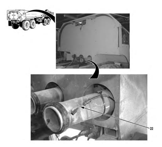
10. Disconnect tank connector (22) from existing chassis harness.
