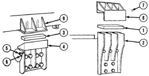
Install two rubber pads (3) on two rear frame mounting brackets (4). Soldier A holds eight screws (5) on two rear frame mounting brackets (4) while Soldier B loosens nuts (6).
