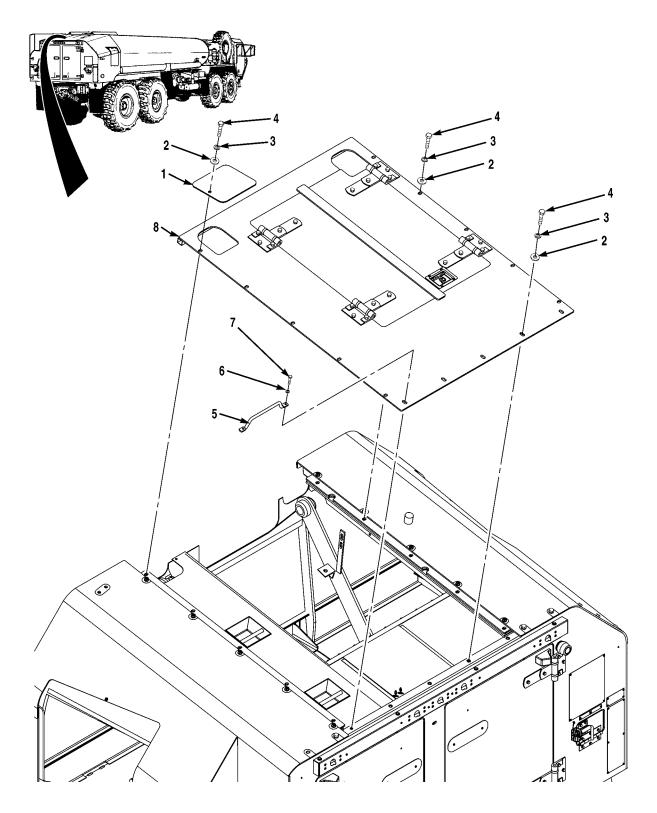
FIG. 6 TOP PANEL ASSEMBLY (SHEET 1 OF 2)
