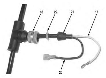
9. Remove rubber seal (21), plastic washer (22), and compression nut (18) from black wire (20) and white wire (17).
