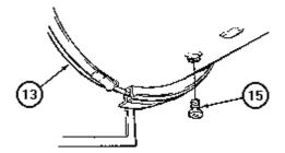
Coat drain plug (15) with pipe thread sealing compound and install plug in fuel tank (13).
