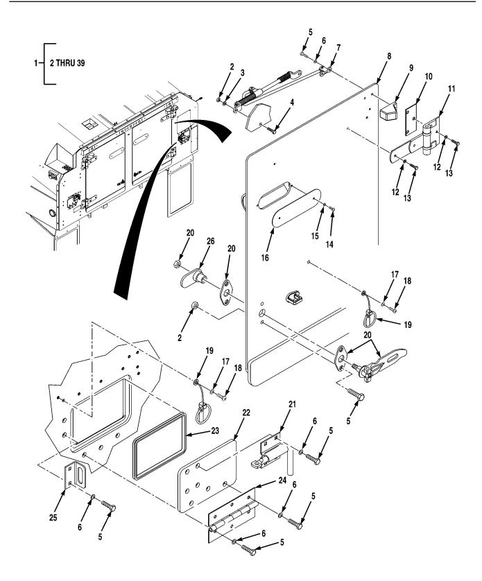
FIG. 1 REAR PANEL ASSEMBLY (SHEET 1 OF 3)
