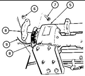
Remove two nuts (6), screws (7), and coupling halves (8) from suction pipe (9) and pump (5).
