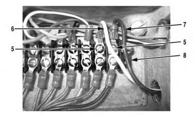
2. Loosen two screws (5) and remove the white wire with brown tape (6) and black wire (7) from terminal board (8).
