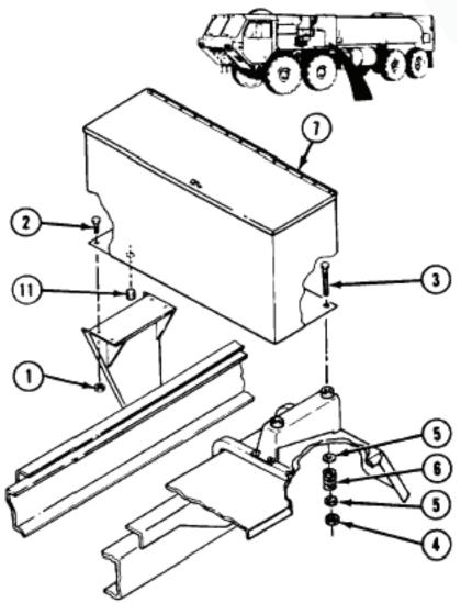
Soldier A operates lifting device and removes stowage box (7) guided by Soldier B. Remove two rubber mounts (8).
