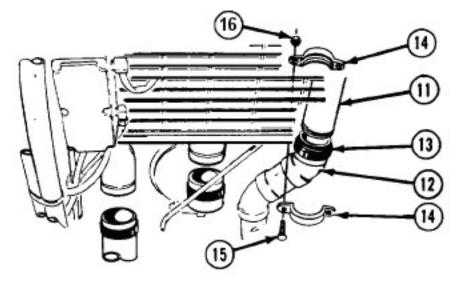
Install two coupling halves (14) on coupling gasket (13) with two screws (15) and nuts (16).
