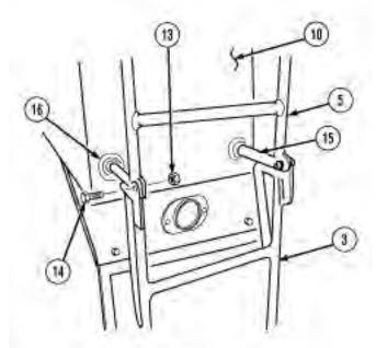
Use cutting wheel and angle grinder to remove ladder supports (15) at pump module (10) and remove upper ladder assembly (5) from pump module (10).
