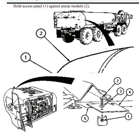
Remove three screws (3) and lockwashers (4). Remove access panel (1) from pump module (2).
