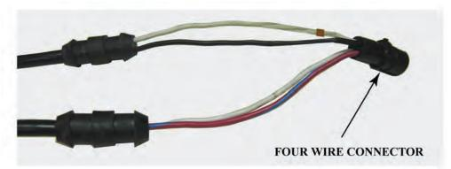
15. Route four wire connector through pump module along the pipe that is farthest toward the driver's side of vehicle. Secure it adjacent to the single brown wire with cable ties, approximately even with the end of the pipe, as shown. Connect four wire connector to matching connector end on existing chassis harness.
