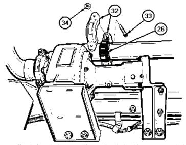
Install two coupling halves (32) on coupling gasket (26) with two screws (33) and nuts (34).
