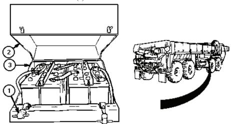
Remove battery box cover (2) from battery box (3).
