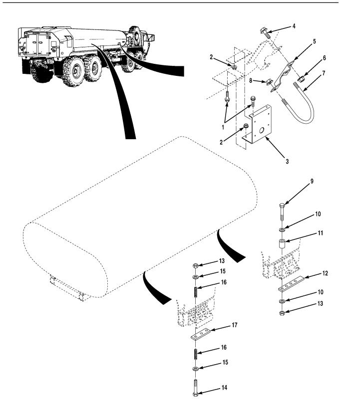
FIG. 9 LADDERS AND BRACKETS (SHEET 1 OF 3)
