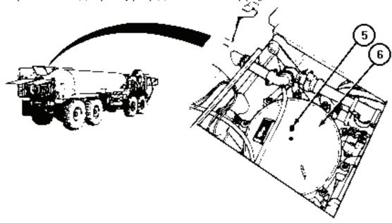
4. Remove plug (5) from filter-separator cover (6).
