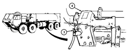
3. Open drain valve (3) in primary pump (4) to drain fuel from piping.
