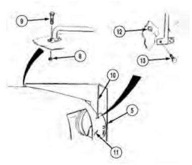
Remove two locknuts (8) and screws (9) from ladder rail (10) and pump module (11). Remove two locknuts (12), screws (13), and ladder rail (10) from pump module (11). Remove ladder rail (10) from bolt-on ladder assembly (5).
