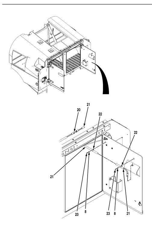
FIG. 8 TANKER MODULE LIGHTING HARNESS ASSEMBLY (SHEET 2 OF 3)
