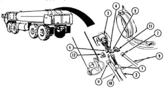
Remove two nuts (7 and 8) and tubes (9 and 10) from elbows (11 and 12). Remove two nuts (13) screws (14) and coupling halves (15) from coupling gasket (16).
