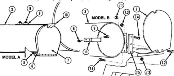
5. Remove two nuts (8) and screws (9) to detach spring catch (10) from stowage tube (3).
