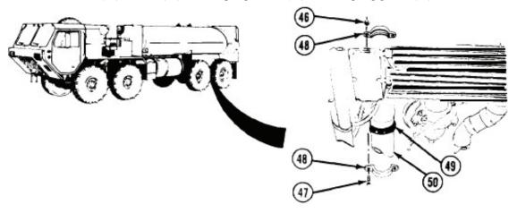
Push coupling gasket (49) onto pipe (50). Remove two nuts (51), screws (52), and coupling halves (53) from coupling gasket (54).
