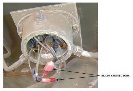
7. Remove nut and conduit tube from center adapter. Pull wires from conduit through adapter. Remove center adapter from compartment light base.
