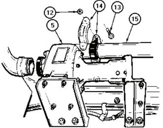
Push coupling gasket back onto discharge elbow.
