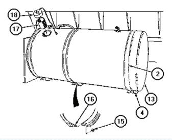
Some models of fuel tanks contain a socket head pipe plug.
