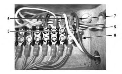
6. Install black wire (7) and white wire with brown tape (6) on terminal board (8) with two screws (5).
