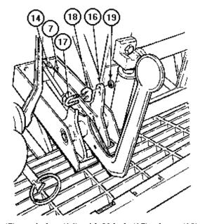
Connect cable (7) to trip bar (16) with U-bolt (17), clamp (18), and two nuts (19).
