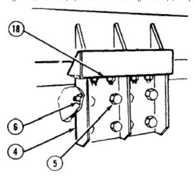
Soldier A holds eight screws (5) while Soldier B tightens nuts (6) behind rear frame mounting bracket (4).
