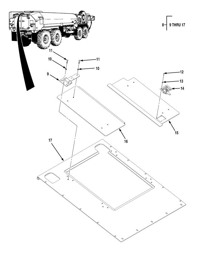
FIG. 6 TOP PANEL ASSEMBLY (SHEET 2 OF 2)
