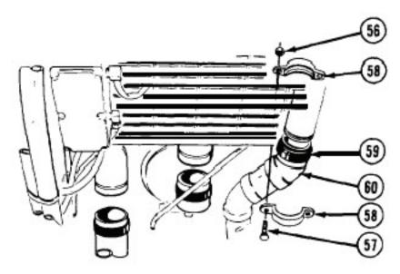
Push coupling gasket (59) onto pipe (60).
