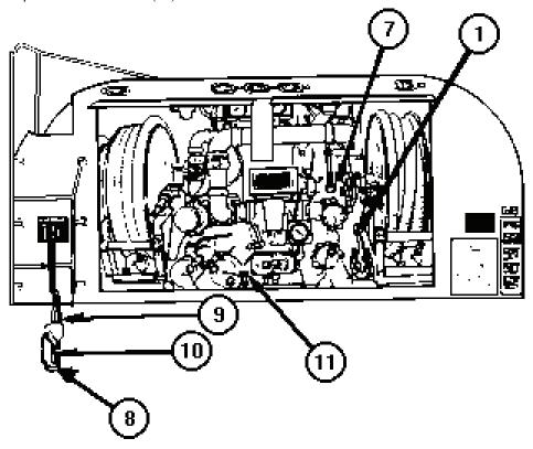
8. Open V15 DRAIN VALVE (11). Remove filter-separator elements.
