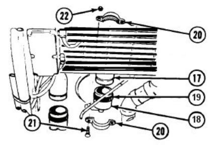
Install two coupling halves (20) on coupling gasket (19) with two screws (21) and nuts (22). Align pipes (23 and 24) and install coupling gasket (25) over connections of pipes.
