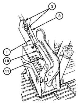
Install cable (1) in offset link (10) with nut (11).
