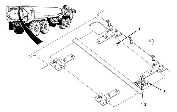
1. Remove four screws (1), lockwashers (2), and one roof door latch assembly (3) from right roof door assembly (4). Discard lockwashers.
