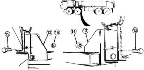
Soldier A removes three screws (15) from right side of tank front crossmember (13) while Soldier B holds and removes locknuts (16).
