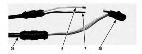
1. Locate four wire connectors (28) on replacement wire harness (26). Cut black wire (7) and white wire with brown tape (6). Discard four wire connector (28) and remaining short end of replacement harness.
