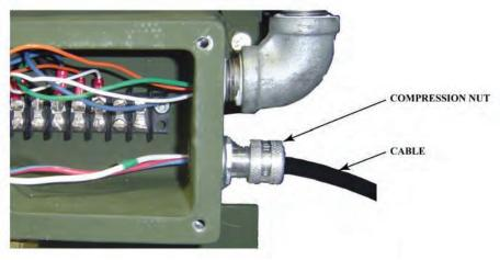
5. Remove rubber seal, plastic washer, and compression nut from wires.
