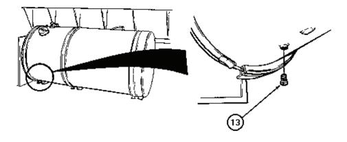
Remove drain plug (13), and drain fuel into container.
