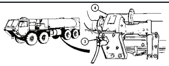
14. Close drain valve (3) on primary pump (4).
