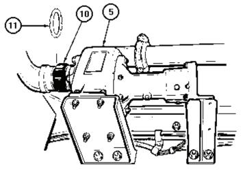
Push coupling gasket (10) onto pump (5). Remove reducer (11) from coupling gasket (10). Remove two nuts (12), screws (13), and coupling halves (14) from discharge pipe (15) and pump (5).
