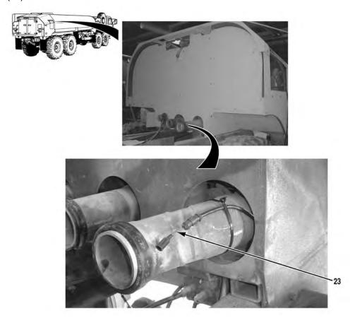
10. Disconnect tank connector (23) from existing chassis harness.
