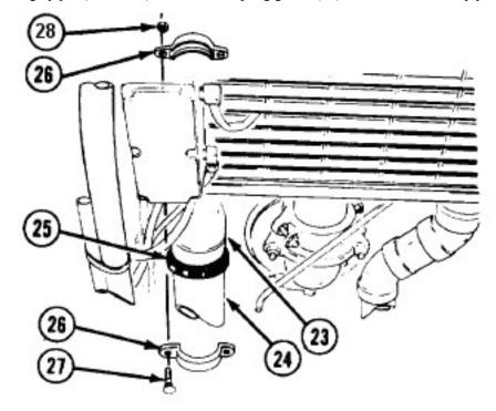
Install two coupling halves (26) on coupling gasket (25) with two screws (27) and nuts (28).
