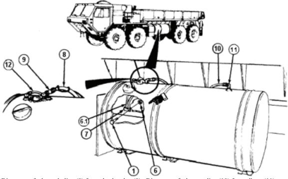
Disconnect fuel supply line (8) from check valve (9). Disconnect fuel return line (10) from elbow (11). Drain fuel from lines (8 and 10) into suitable container.
