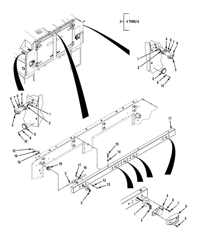
FIG. 8 TANKER MODULE LIGHTING HARNESS ASSEMBLY (SHEET 1 OF 3)
