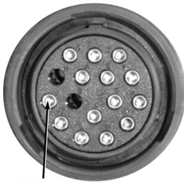
TERMINAL J WIRE 1630
