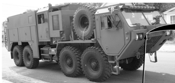
PASSENGER SIDE FRONT LOWER WARNING LIGHT
