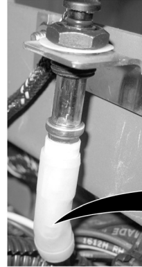
DRIVER SIDE STOWAGE HATCH DOOR SWITCH WIRE 1474 WIRE 2460
