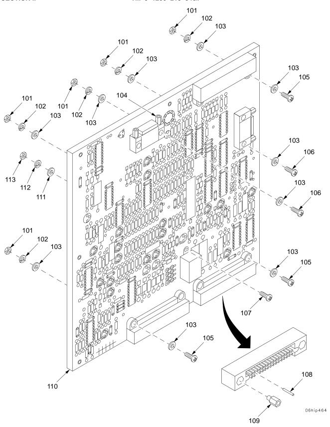
Figure C13. Circuit Card Assembly, PCU Main (12561695) (Sheet 3 of 3)
