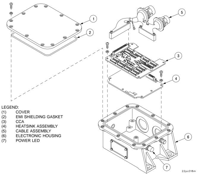
Figure 5-3. VMS Modem Exploded View
