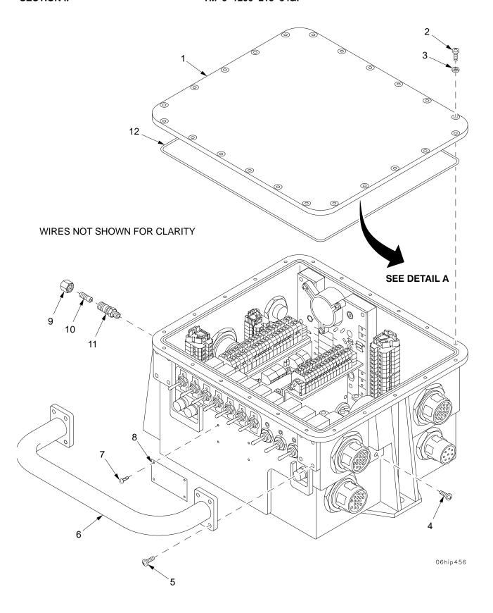
Figure C11. Control, Power Supply (12561743) (Sheet 1 of 20)
