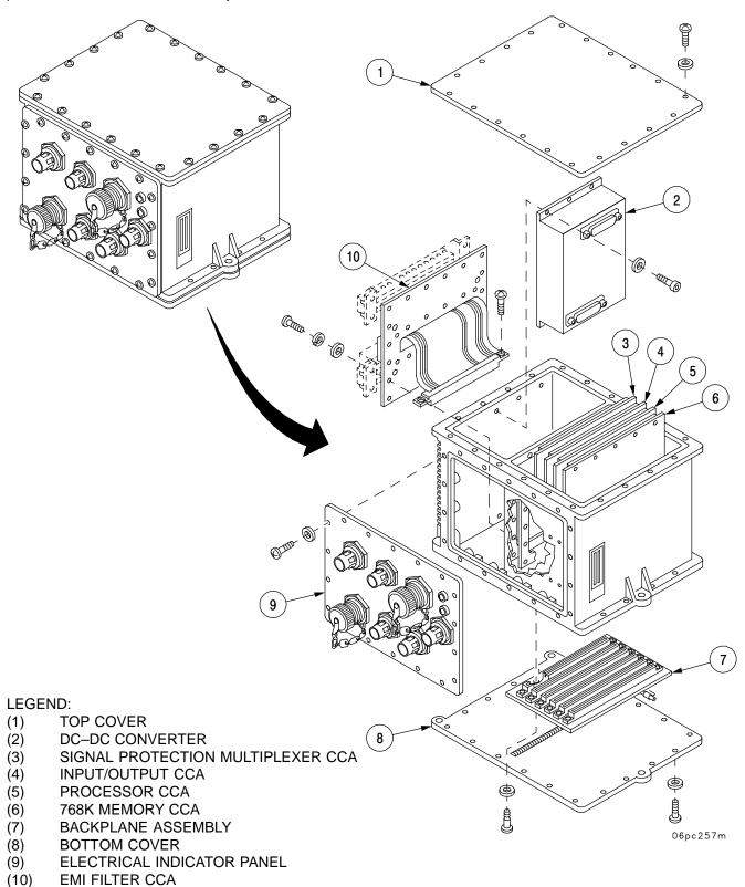
d. The VMS Modem is comprised of an aluminum casting electronic housing, modem circuit card assembly, power supply, heatsink assembly, and cable assembly. The location of these components is shown in the following illustration:
