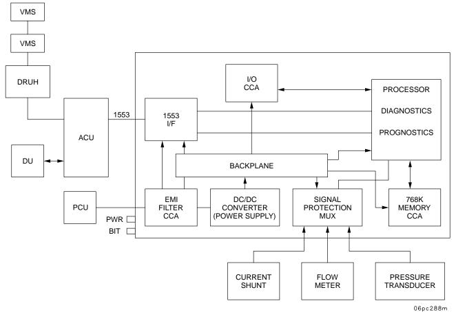
Figure 4–1. Prognostic/Diagnostic Interface Unit Block Diagram
