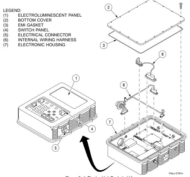
Figure 3-4. Display Unit Exploded View
