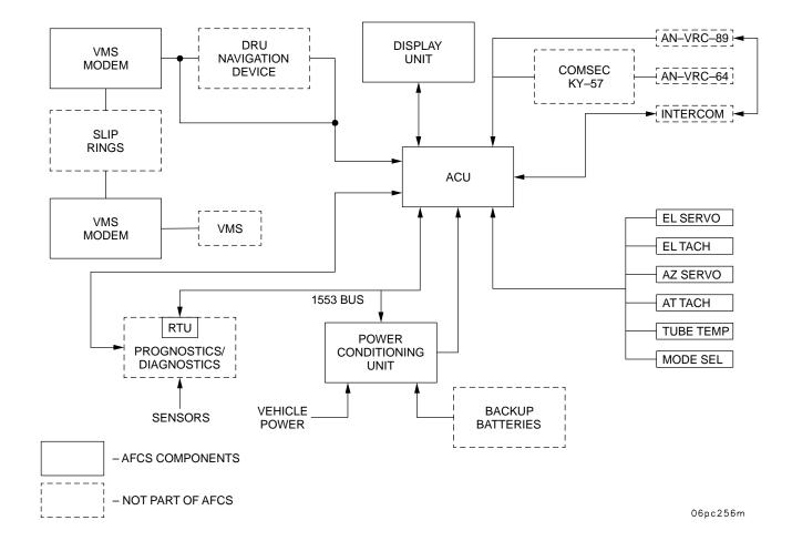
Figure 1-1. AFCS Block Diagram
