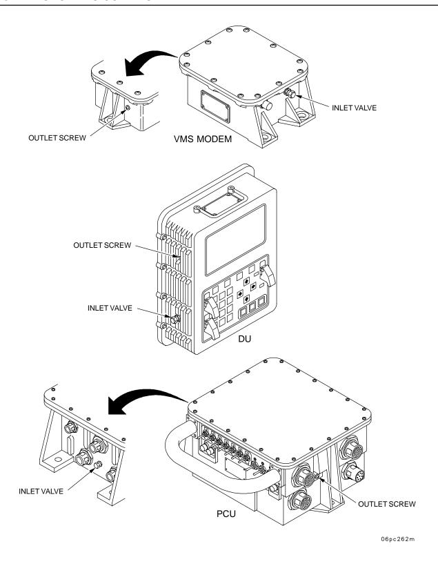
Figure 1–2. Location of Inlet Valves and Outlet Screws on AFCS LRUs
