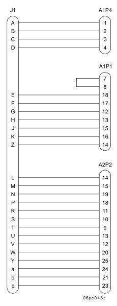
Figure 3-3. DU-Serial Cable Assembly
