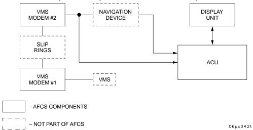
Figure 5-1. VMS Modem Block Diagram
