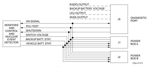
Figure 6-5. Status Monitor Circuit and Nuclear Event Detector Interface Diagram
