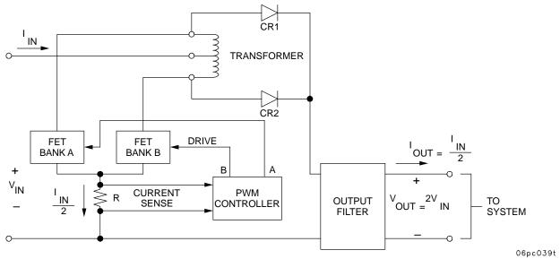
Figure 6-3. Voltage Doubler Block Diagram
