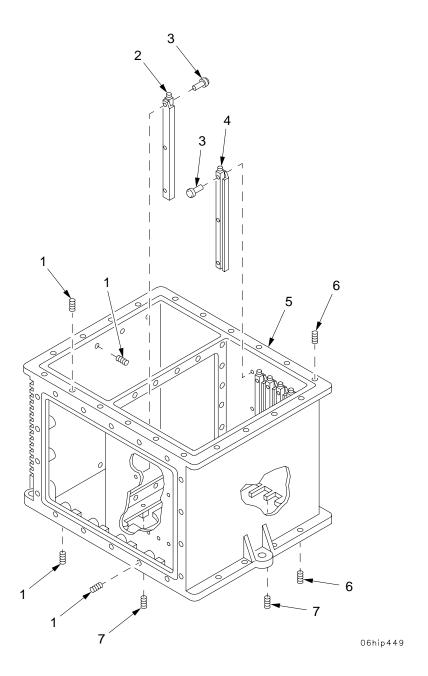
Figure C9. Chassis, Electronic (12562738)
