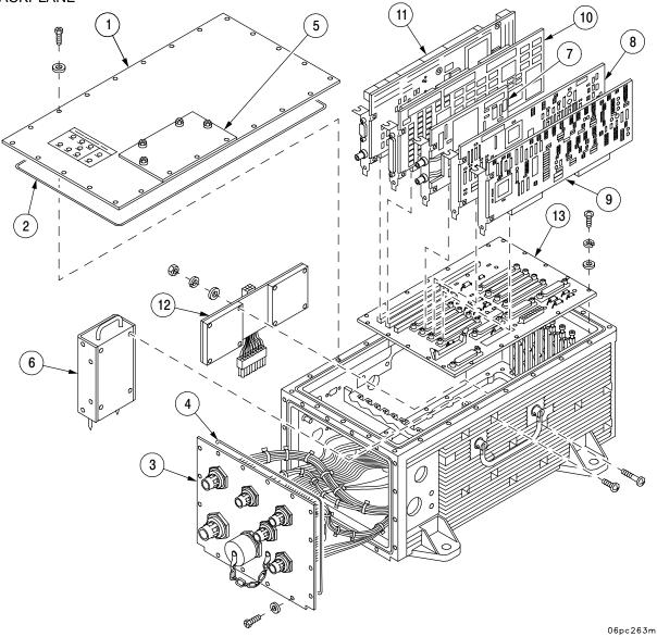
Figure 2-3. AFCS Control Unit Exploded View
