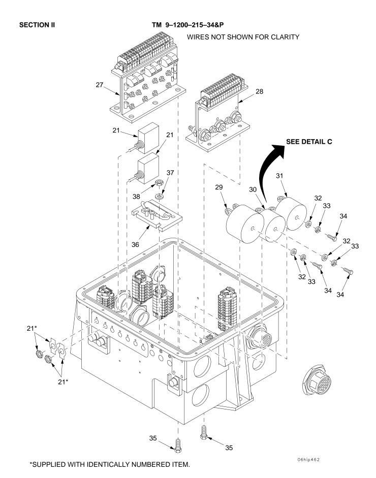
Figure C11. Control, Power Supply (12561743) (Sheet 4 of 20)
