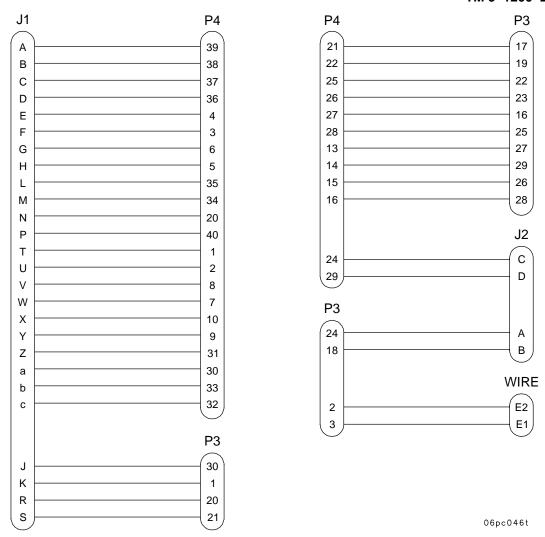
Figure 5-2. VMS Cable Assembly
