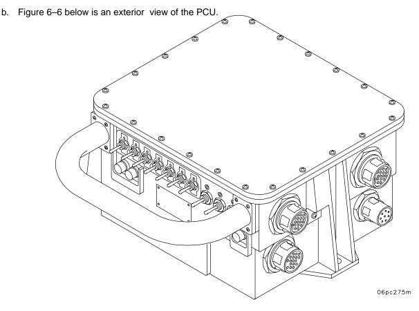
Figure 6-6. Power Conditioning Unit
