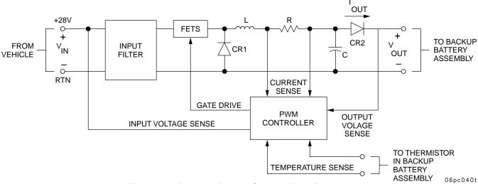
Figure 6-4. Back-up Battery Charger Block Diagram
