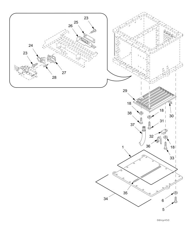
Figure C4. Prognostic/Diagnostic Interface Unit (12554020), Cover, Access (12554022), Cover, Access (12562726) (Sheet 2 of 2)
