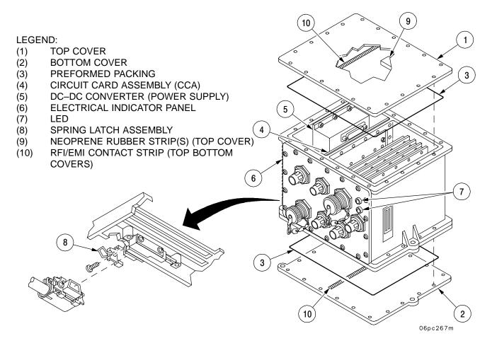
Figure 4–2. PDIU Exploded View
