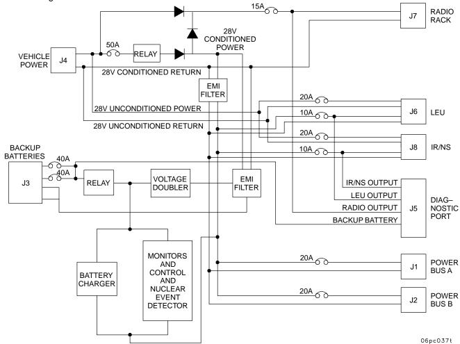
Figure 6-1. PCU Block Diagram
