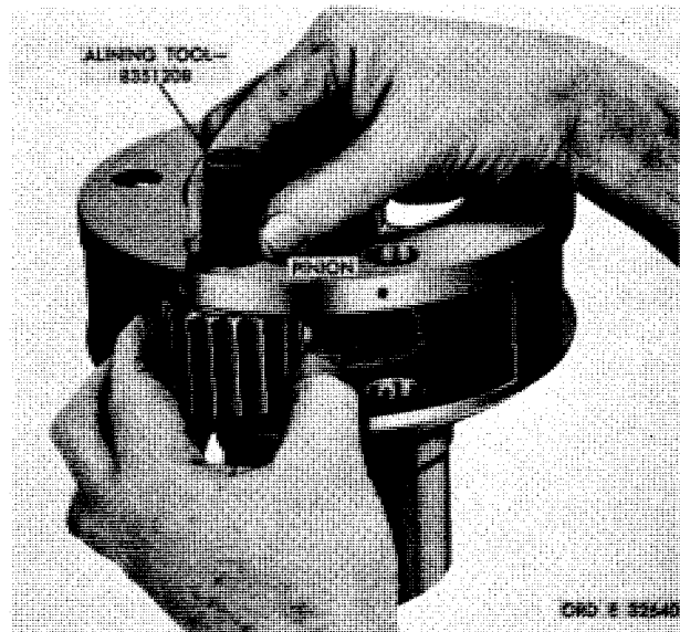
Figure 221. Alining pinion and component parts in planetary carrier
