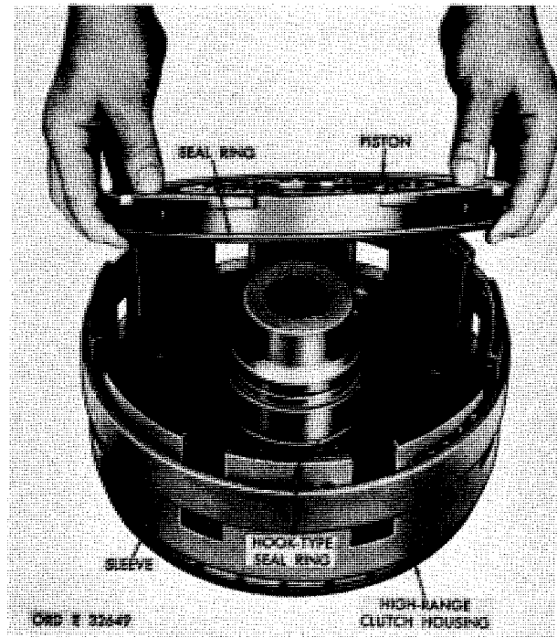
Figure 230. Removing (or installing) piston from high-range clutch housing
