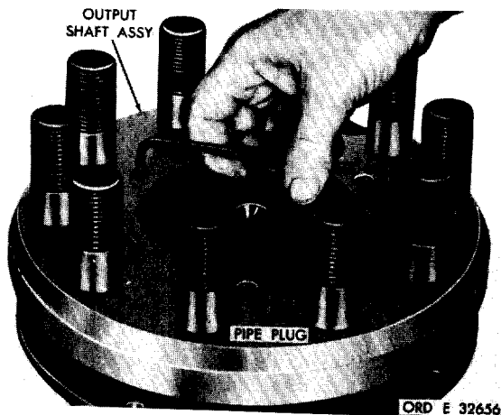
Figure 237. Removing pipe plugs from output shaft assembly
