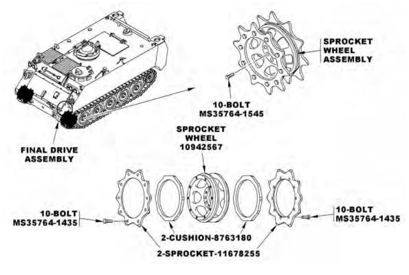
Figure 2. Remove One T130E1 Track Assembly and Sprocket Wheel Assembly from Vehicle
