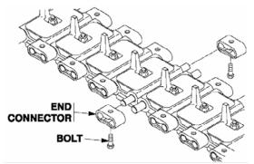
Figure 4. Install T150F Track Assembly on Vehicle
