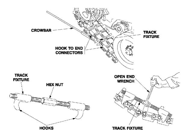
Figure 5. Install T150F Track Assembly on Vehicle
