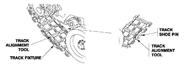
Figure 6. Install T150F Track Assembly on Vehicle
