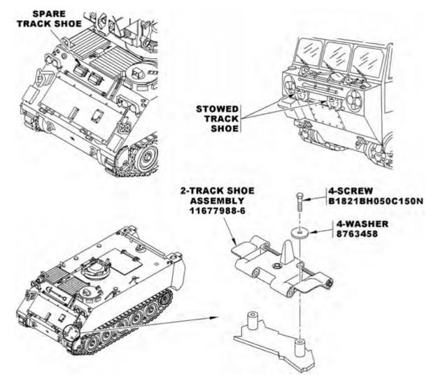
Figure 1. Remove Stowed Track Shoe Assemblies
