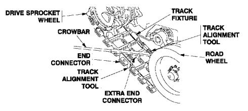
Figure 8. Install T150F Track Assembly on Vehicle
