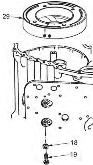
Figure 26. Second Clutch Piston Housing Assembly Installation.
