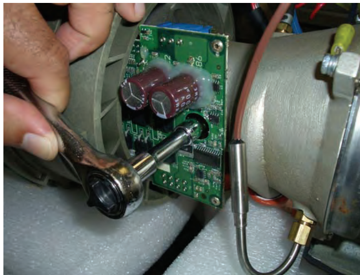
Figure 5.6-7 Bolt Removal Detail, Vent Fan Assembly
