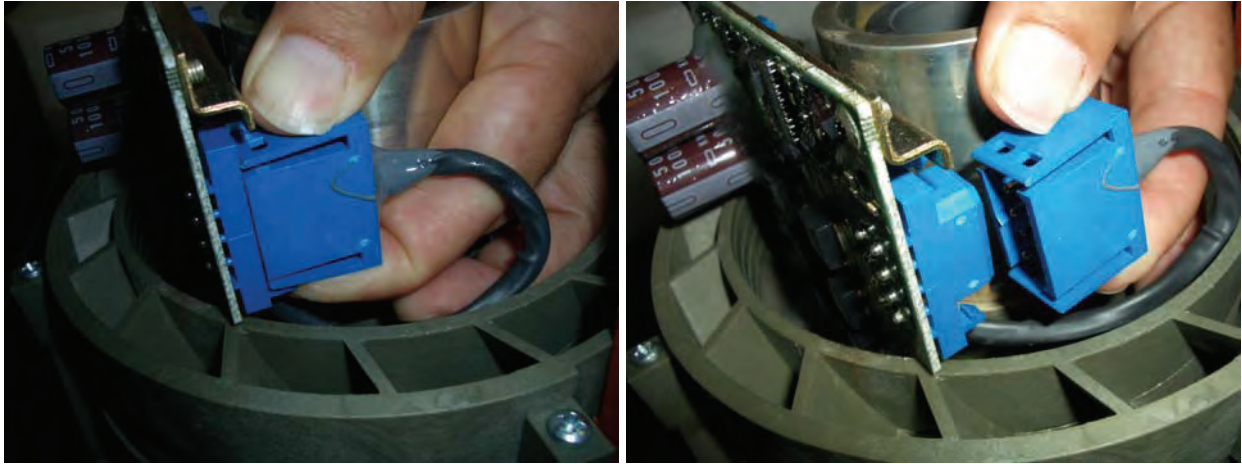
Figure 5.6-21 Detail, Removal of Printed Circuit Board Connector
