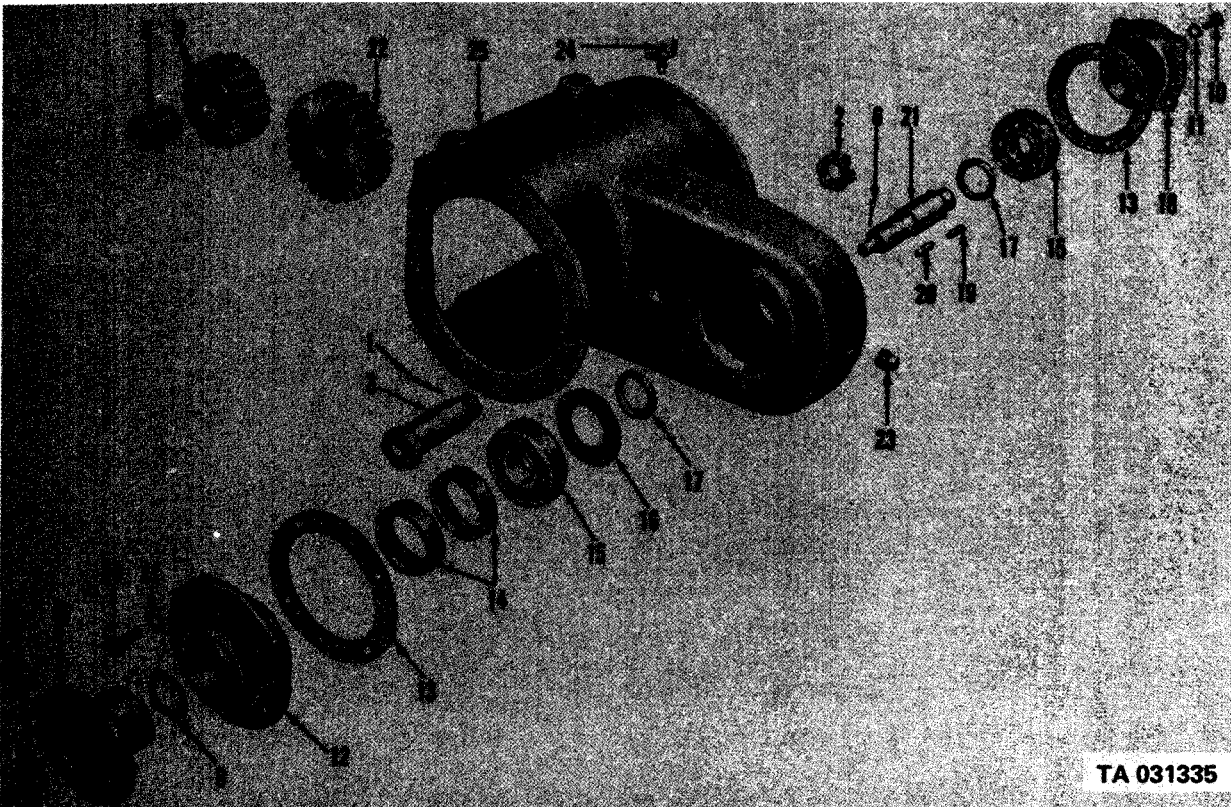
Figure 243. Earth boring machine input gears and shafts (V18A/MTQ).
