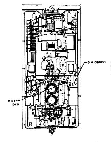
Auxiliary Power Unit Crankcase Fill and Level (See note 77 and view BU) (C)
