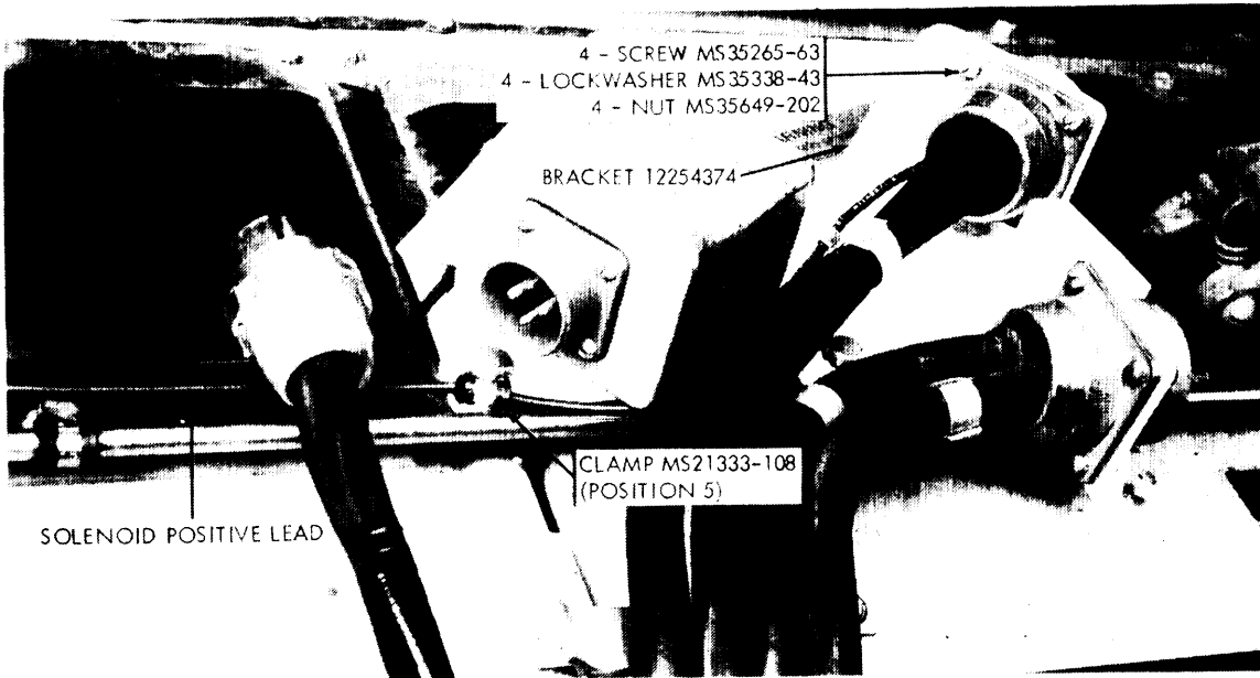
Figure 24. Installation of Solenoid Positive Lead Clamp at Position 5
