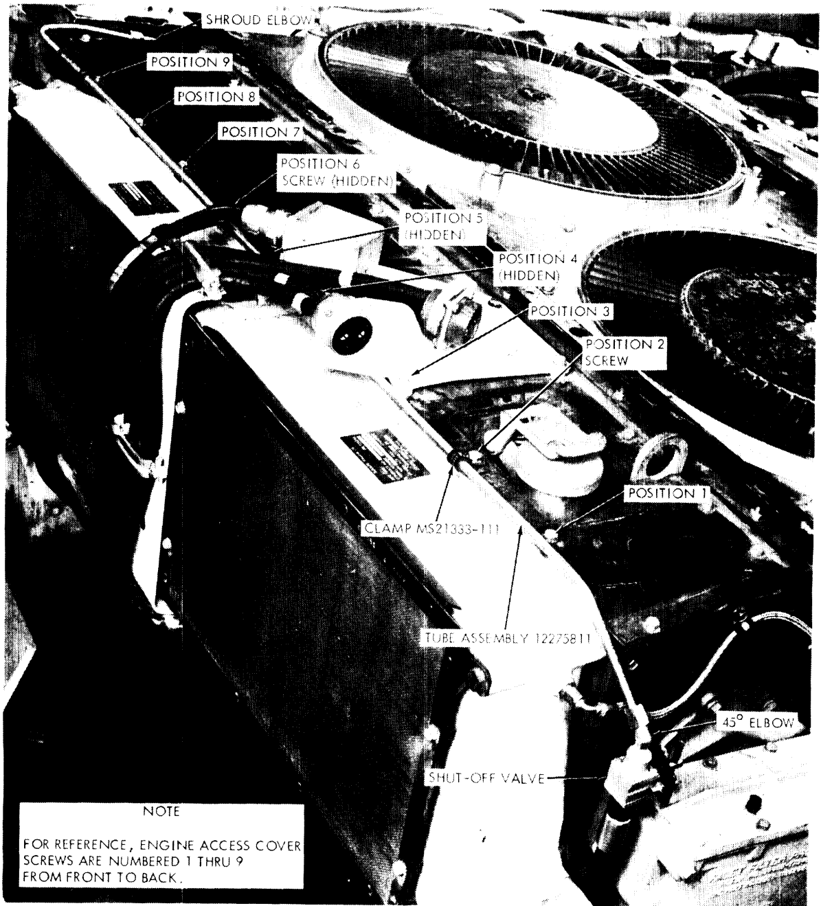
Figure 18. Installation of Tube Assembly 12275811
