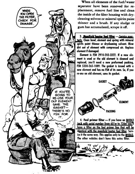
terly. Clean bowl, element and spring with mineral spirits paint thinner or drycleaning solvent. Blow dirt out of element with compressed air. Replace
