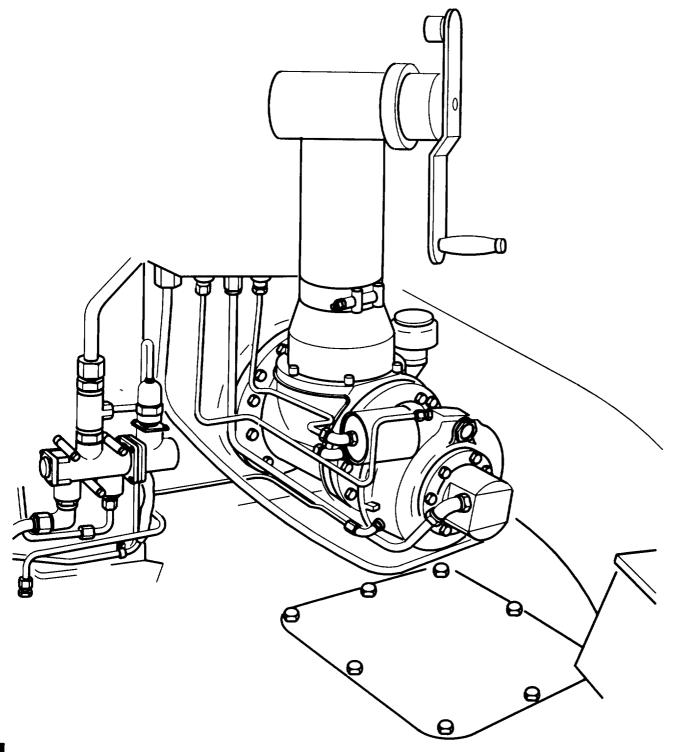
Figure 10-1.1. Manual Elevating Hand Pump (M 110 series only)
