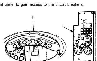
M110/M578 Master Switch Panel (1) and Instrument Panel (2)
