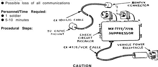
Without the transient voltage suppressor in the circuit, voltage spikes will be routed through the communications equipment and damage could occur. Use only as a last resort.
