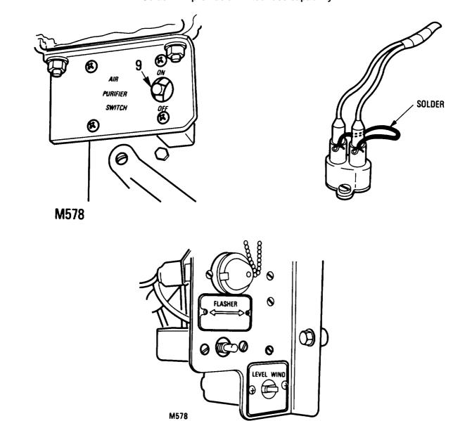
4. Connect the electrical wires together by inserting a piece if solder or insulated wire in the connector plugs or cut wires and twist together.
