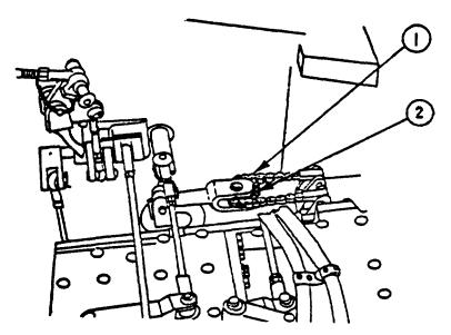
2. Remove broken pieces of chain (item 1) from around sprocket (item 5), if any.
