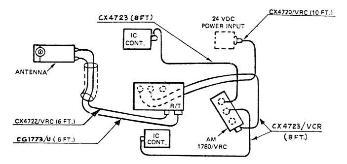
NOTE: THERE IS A 40 FT. AUDIO EXTENSION CABLE AND RF CABLE BETWEEN THE MX-6707 AND THE R/T.
