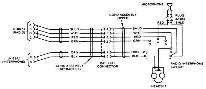
CVC HELMET (Headsel-Microphone Kit MK-1697-G, wiring diagram.)
