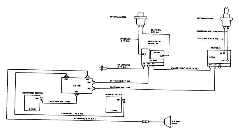
AN/VRC-46, AN/VRC-64, or Two AN/GRC-160's (Turret) vith AN/VIC-1 ⊒. **M**2 and Μ3
