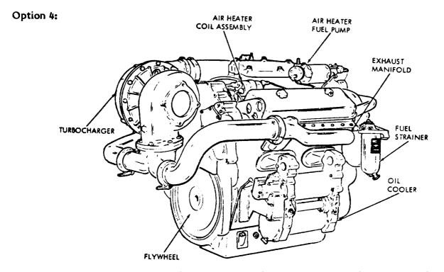
Figure 3-4. Engine Assembly (Model 7083-7398) Right Rear View (Early Version)
