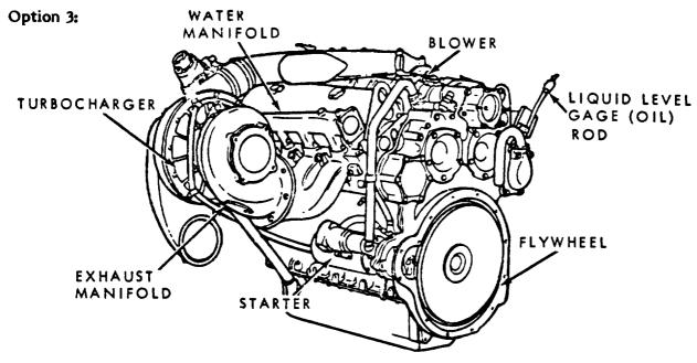
Figure 3-3. Engine Assembly (Model 7083-7396) Left Rear View
