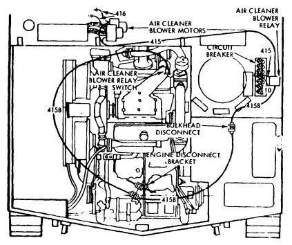
2. Locate air cleaner blower relay behind portable operators panel in driver's compartment.
