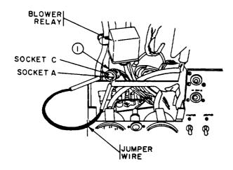
4. Using jumper lead connect sockets A and C together. The jumper lead must be wedged into the female sockets of connector to prevent them from vibrating out of the sockets.
