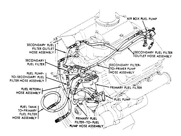
Fig 3-7. Engine fuel system.
