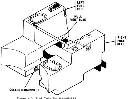
Figure 4-2. Fuel Cells for M110/M578
