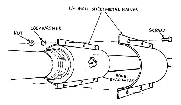
8. Secure bands against bore evacuator with screws, nuts, and lockwashers.
