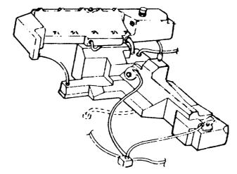
Figure 4-1. Fuel Storage Tank for M109
