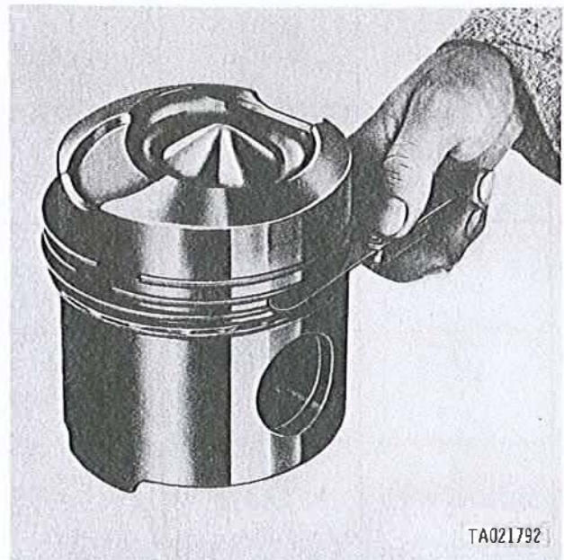
Figure 3-184. Checking piston ring side clearance.
