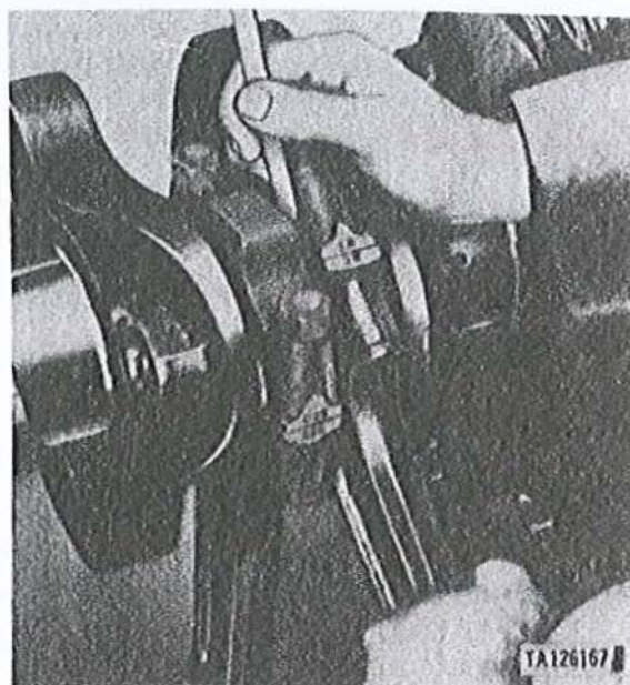
Figure 3-176. Checking connecting rod side clearance.
