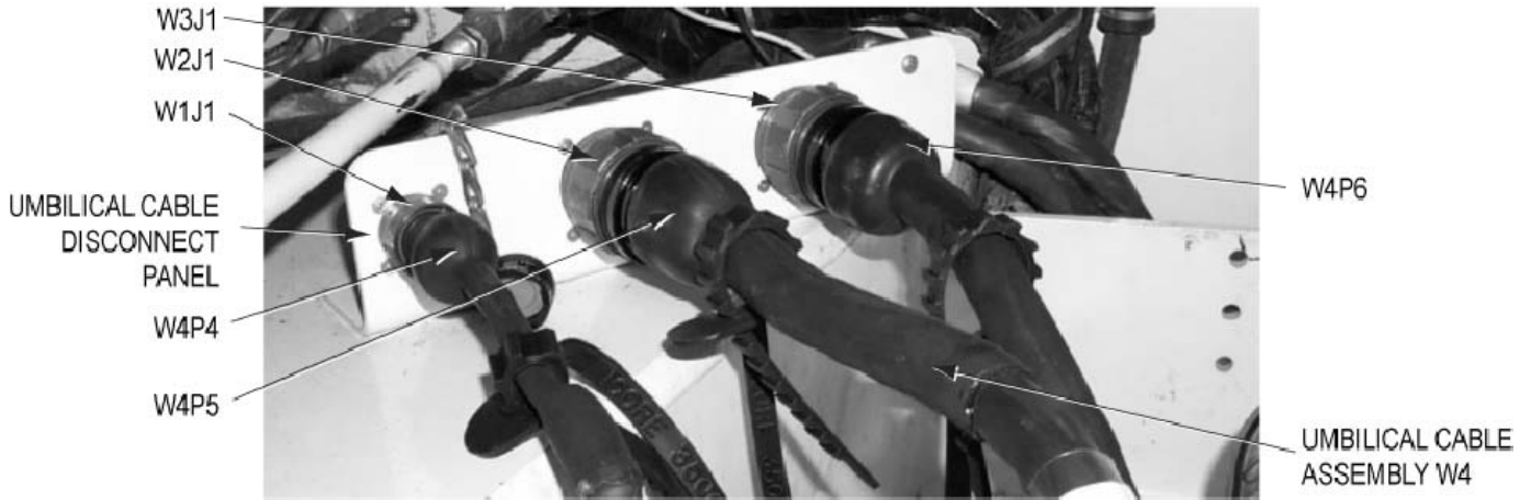
Figure 5-20. Umbilical Cable Assembly W4 Connection to Umbilical Cable Disconnect Bracket
