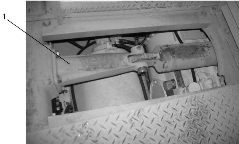
Figure B-5. Ejector Cylinder Bracket Removal
