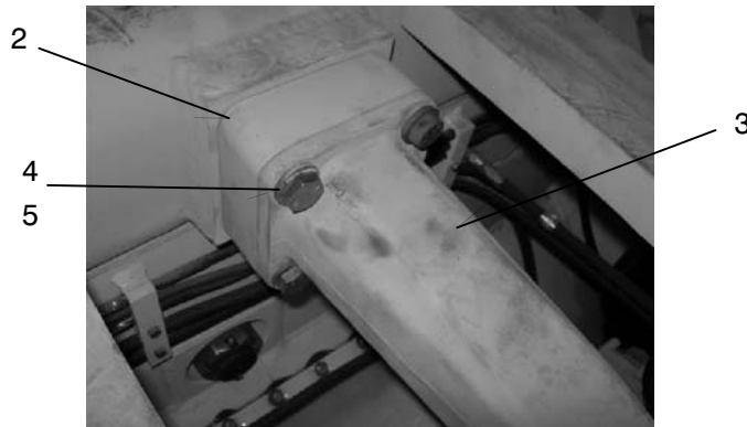
Figure B-6. Spacer Block Installed
