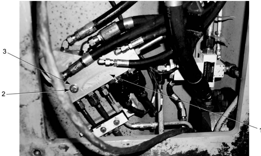
Figure 4-4. Installation of New Forward Left Manifold Assembly
