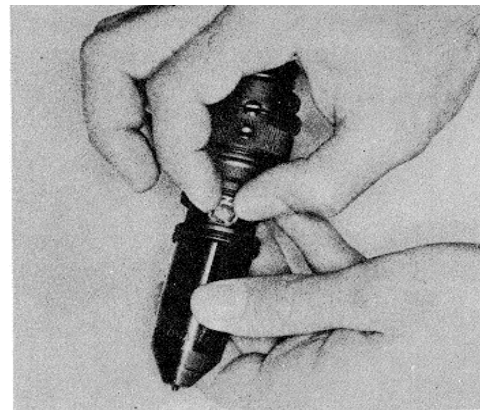
Fig. 6-1-42, F60202. Fuel inlet screen and retainer
