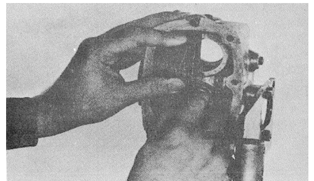
Fig. 5-20, F5136. Scribe center line on fuel pump housing
