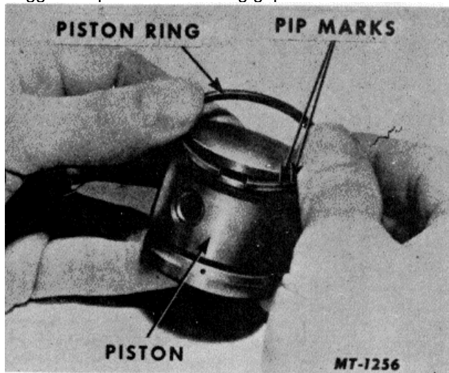
Fig. 11 Installing Piston Rings
