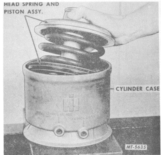
Fig. 13 Removing Head, Spring and Piston Assembly
