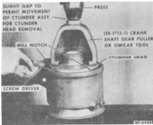
Fig. 12 Using Screwdriver to Loosen Cylinder Head
