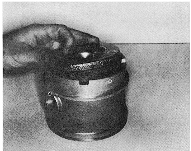
Fig. 10-22, T-529. Installing insulation pad
