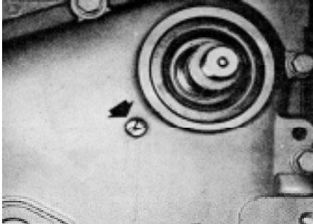
Fig. 14-22, (N114143). Camshaft and accessory drive gear timing marks
