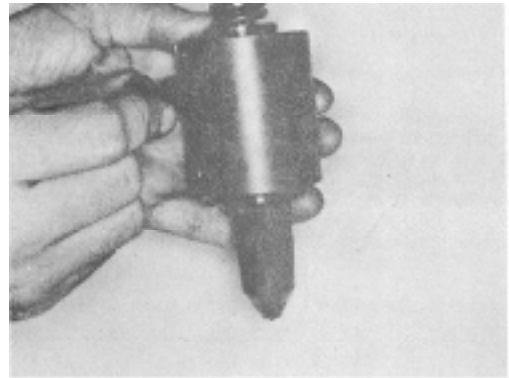
Fig. 6-1-110, F60212. Tighten ST1058 locating screw
