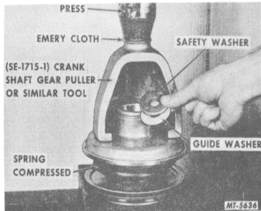
Fig. 15 Removing Safety Washer and Guide Washer.
