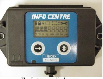
The first screen displays an all Segment Display Test
