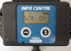
If display is other than 07, reference pages 5-7. Repair, re-power and clear stored faults again.
