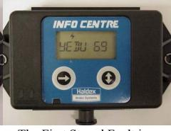
The First Stored Fault is Displayed. Example: "Yedu 69" Fault
