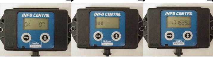
From the Active Fault screen, Code 07, Vehicle is Stationary.
