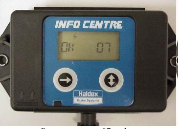
Powers up to an 07 code, Vehicle is Stationary. ABS is fully operational. If vehicle ABS Lamp is still On, check stored faults. (see page 2).
