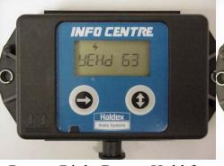
Repeat Right Button Hold for next Stored Fault. Example: "Yehd 63" Fault
