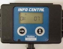
After Clearing Stored Faults, the Display Returns to the Active Fault Screen.
