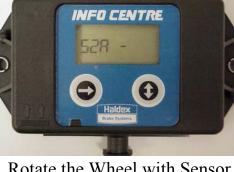
Rotate the Wheel with Sensor 2A (1 rev/ 2 sec) 4 sec min. S2A will remain Displayed
