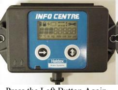
Press the Left Button Again To View Segment Display Test
