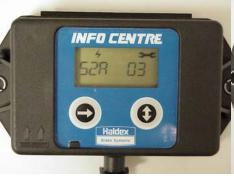
Repeat Right Button Hold for Repeat Right Button Hold until next Stored Fault. Example: "S2A 03" Fault
