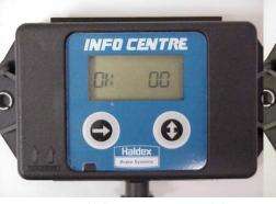
Repeat Right Button Hold to Clear Stored fault Codes. otherwise wait to return to the Active Fault Screen
