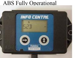
Rotate the Wheel with Sensor 2B (1 rev/ 2 sec) 4 sec min. 2B will remain Displayed
