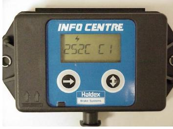
Next screen displays ABS Sensor/Valve Configuration 2S2C C1= (2Sensors/2 Valves)
