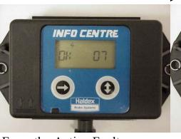
From the Active Fault screen, Code 07, Vehicle is Stationary
