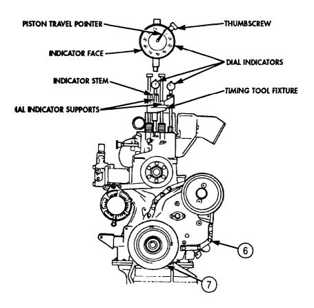
11. Read right hand push tube travel indicator. If push tube travel is not 0.0290 in. (0.74 mm), continue to step 12.
