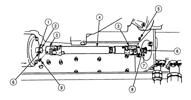
FOLLOW-ON TASK: Start engine (TM 9-2320-272-10) and operate any accessory driven by the transmission PTO-to-hydraulic pump propeller shaft. Stop engine (TM 9-2320-272-10) and check shaft for looseness.
