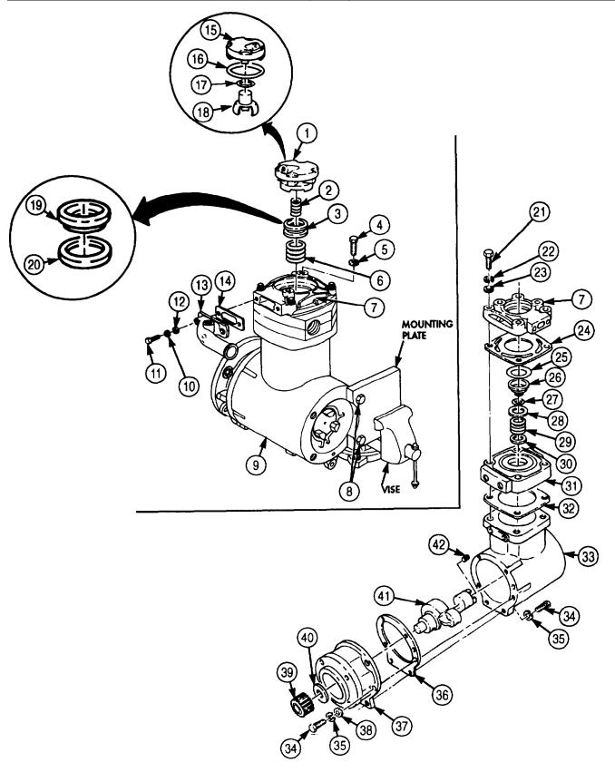
16. Remove piston (7) and connecting rod (8) from crankcase (9).
