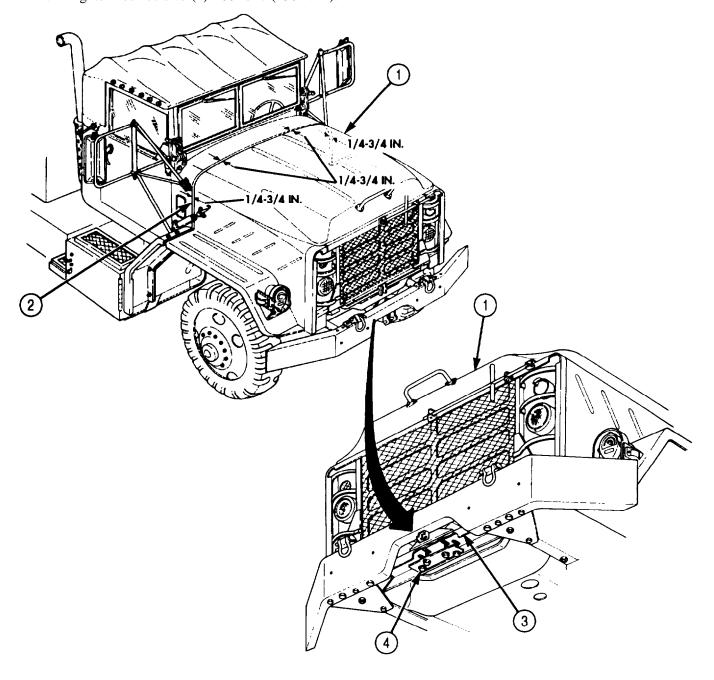
FOLLOW-ON TASK: Install left and right splash shields (TM 9-2320-272-10).
