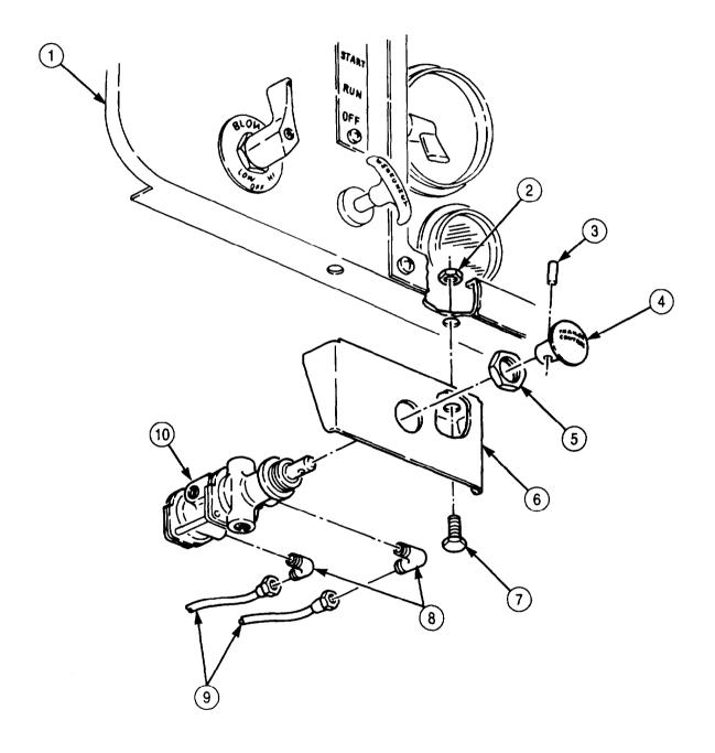
FOLLOW-ON TASK: Start engine (TM 9-2320-272-10) and allow air pressure to build to normal operating range. Check air supply valve for leaks.
