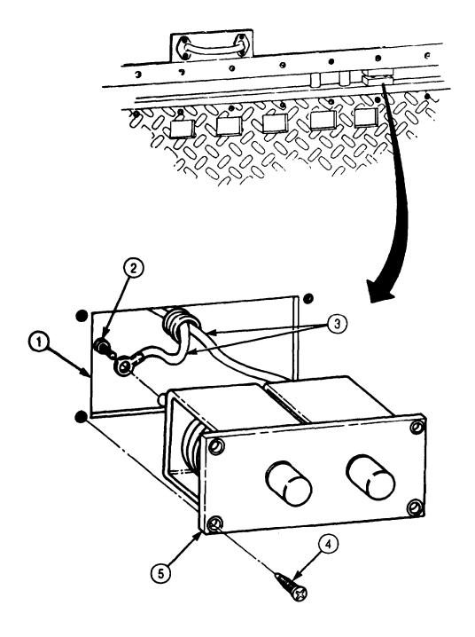
FOLLOW-ON TASKS: Turn on main power switch and check operation of side and rear door blackout switches (TM 9-2320-272-10)
