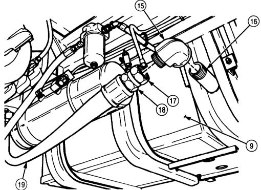
FOLLOW-ON TASKS: •Fill hydraulic oil reservoir to proper fluid level (LO 9-2320-272-12). •Operate hydraulic system (TM 9-2320-272-10) and check for leaks.
