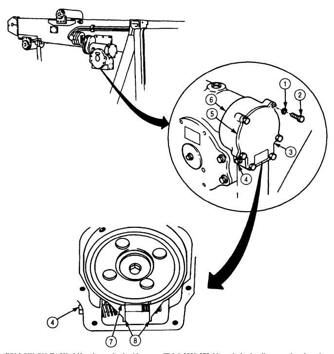
FOLLOW-ON TASK: Lift a heavy load with crane (TM 9-2320-272-10) and check adjustment by observing slippage when trying to sustain load. If crane does not hold load, notify DS maintenance.
