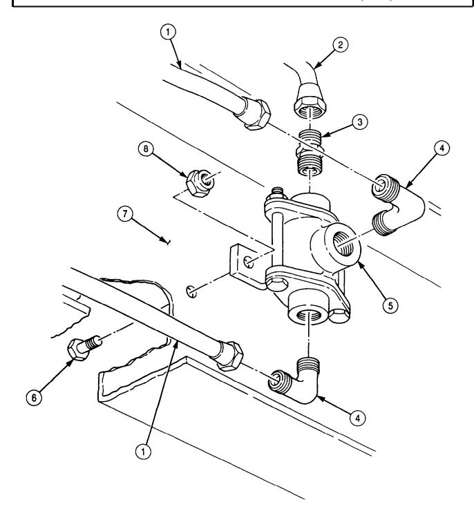
FOLLOW-ON TASK: Start engine (TM 9-2320-272-10) and allow air pressure to build to normal operating range. Check doublecheck valve for leaks.
