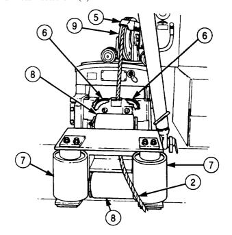
FOLLOW-ON TASK: Wind winch cable on drum (TM 9-2320-272-10).
