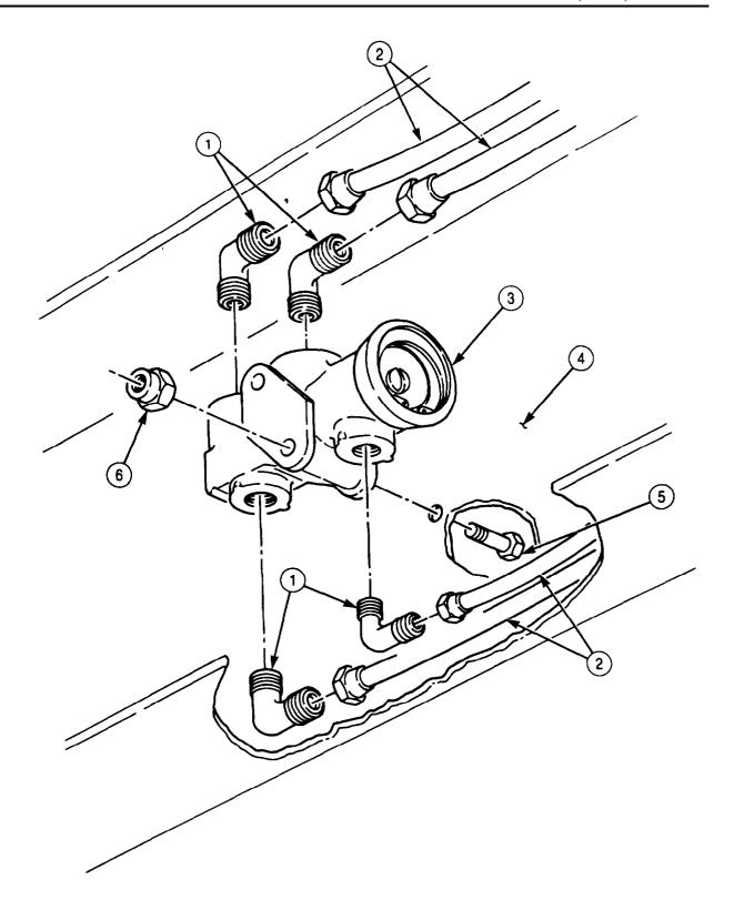
FOLLOW-ON TASK Start engine (TM 9-2320-272-10) and allow air pressure to build to normal operating range. Check valve for leaks.
