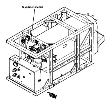
Disconnect cable assembly from sensing elements.
