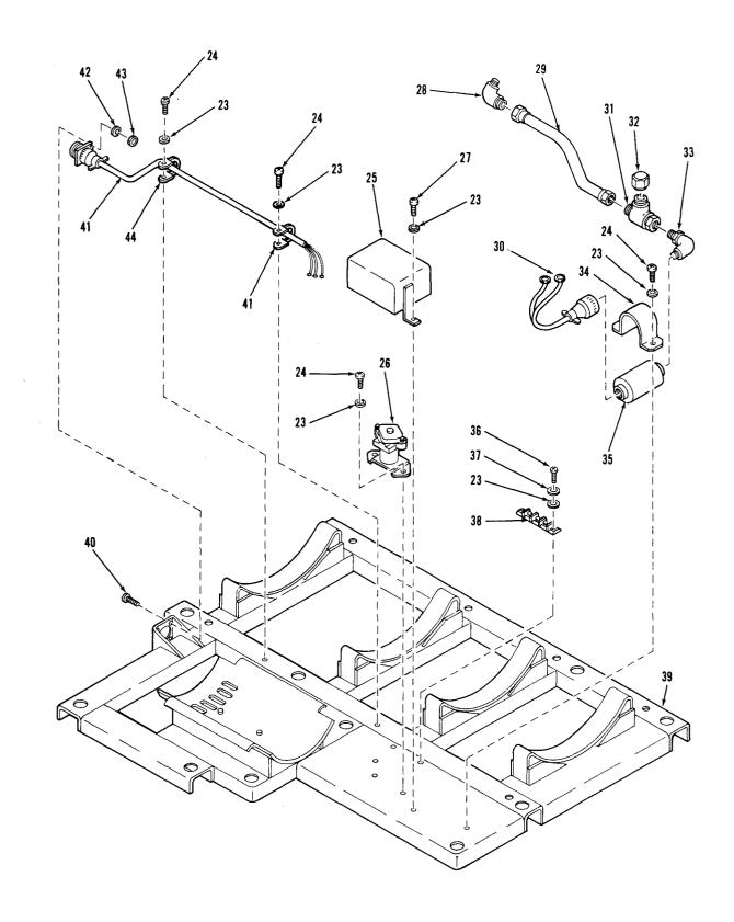
Figure F-21. Air Compressor Assembly (Sheet 2 of 2)
