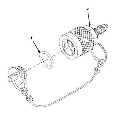
Figure F-5. Quick Disconnect Coupling Half
