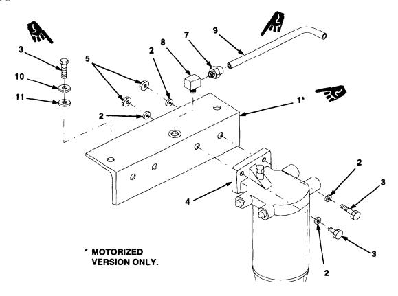
Figure F-27. Fuel Filter/Water Separator Assembly
