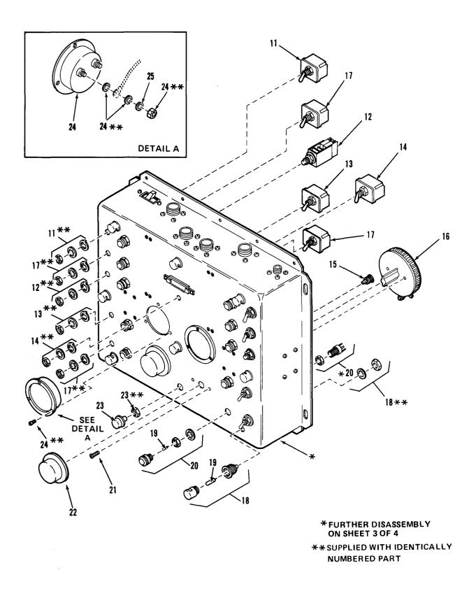
Figure F-16. Control Panel Assembly Panel Cover (Sheet 2 of 4)
