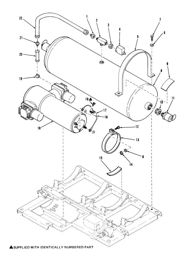
Figure F-21. Air Compressor Assembly (Sheet 1 of 2)
