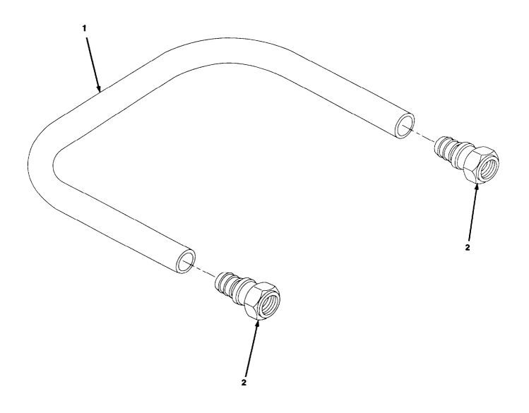
Figure F-4. Fuel Pressure Hose Assembly
