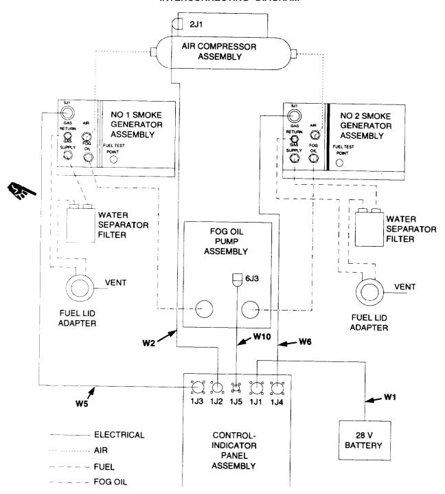
Connect remaining cable and hose assemblies according to the interconnecting diagram. Route cable and hoses behind retaining straps of fog oil tank where possible.
