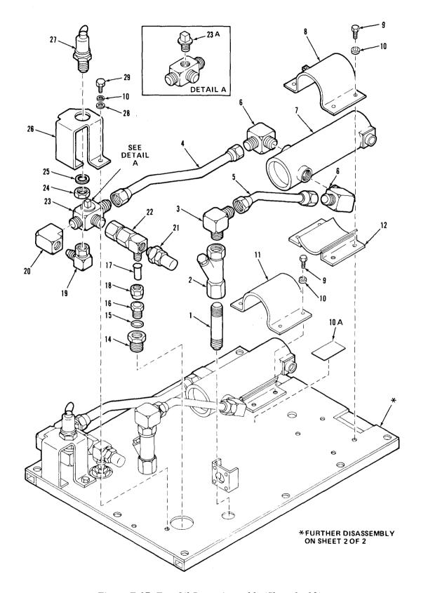
Figure F-17. Fog Oil Pump Assembly (Sheet 1 of 2)
