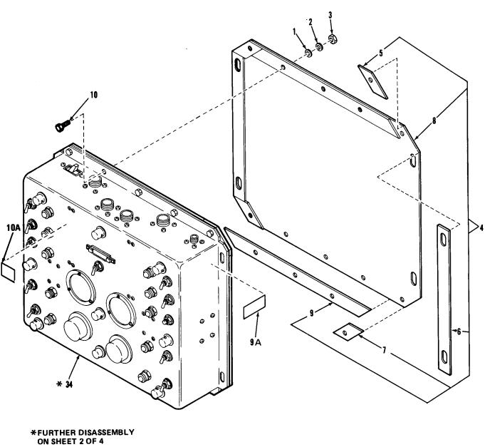
Figure F-16. Control Panel Assembly Panel Cover (Sheet 1 of 4)
