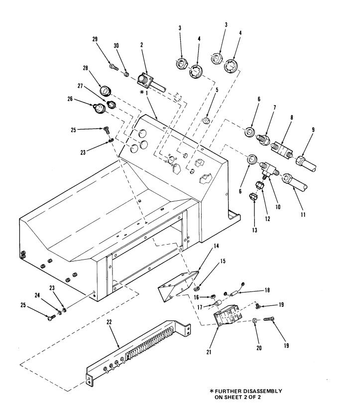
Figure F-6. Equipment Container Assembly (Sheet 1 of 2)
