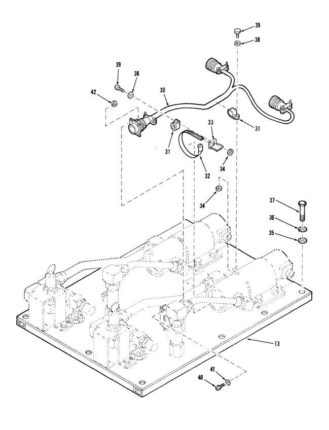
Figure F-17. Fog Oil Pump Assembly (Sheet 2 of 2)
