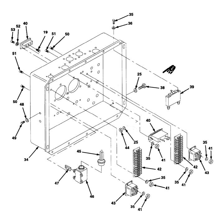
Figure F-16. Control Panel Assembly and Panel Cover (Sheet 4 of 4)
