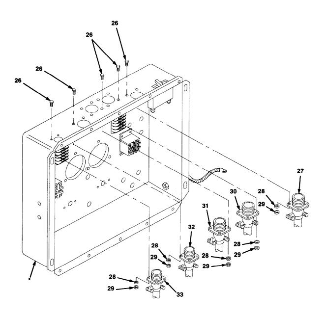
Figure F-16. Control Panel Assembly and Panel Cover (Sheet 3 of 4)
