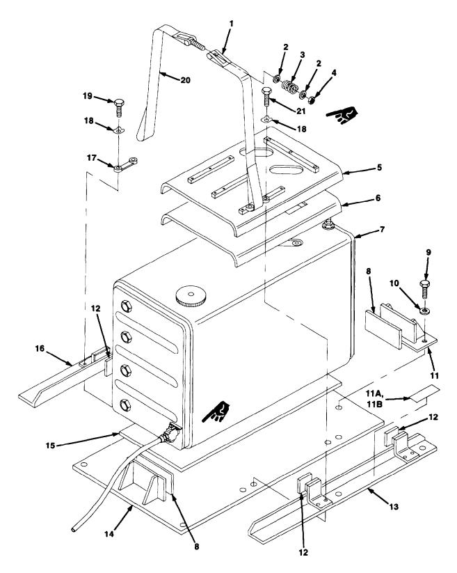
Figure F-25. Fog Oil Tank Assembly
