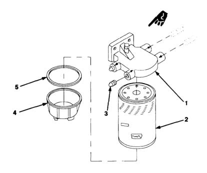
Figure F-28. Fuel Filter/Water Separator
