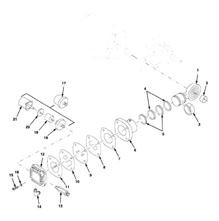
Figure F-23. Compressor Pump Assembly
